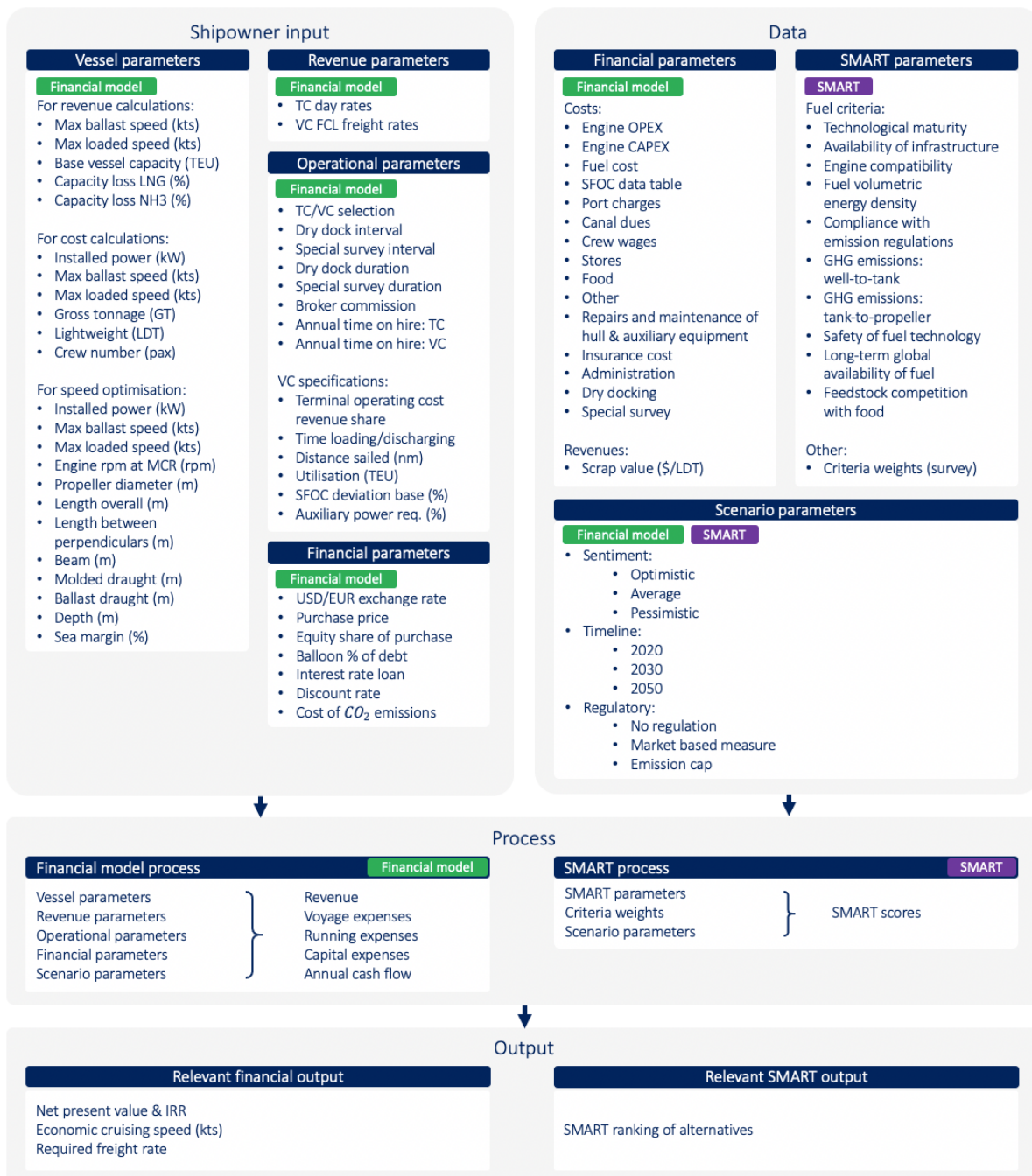
Figure 8.1: Schematic overview of decision tool architecture. Own composition
