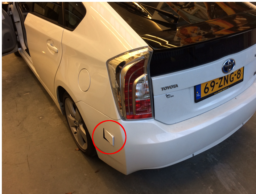
Figure 2.3: Sensor placement position, the rectangular opening around the latch lets air through for measurements by the barometer. The red circle shows the latch behind which the weather sensors are placed.
