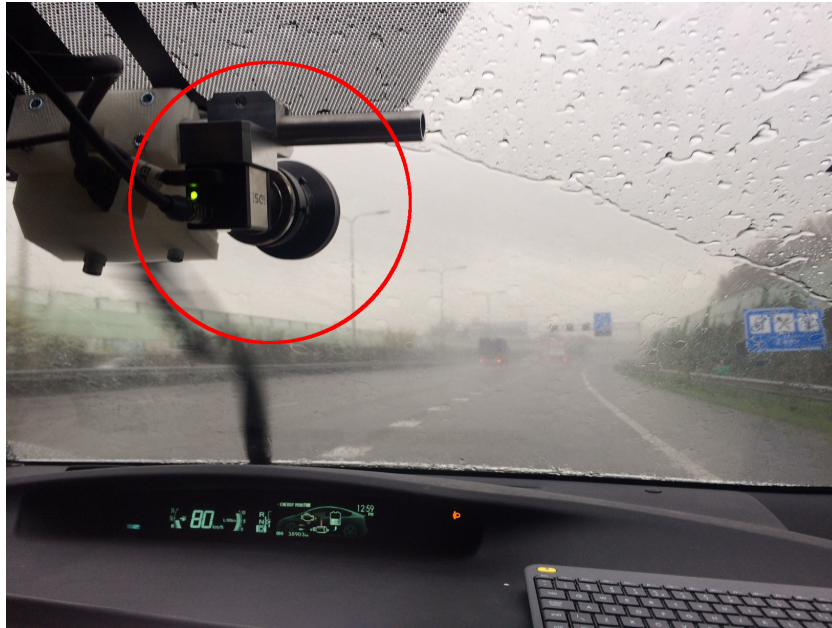
Figure 2.4: Interior photo showing camera placement. The red circle indicates the camera location. The camera orientation is horizontally and vertically level. Image taken from passenger side.
