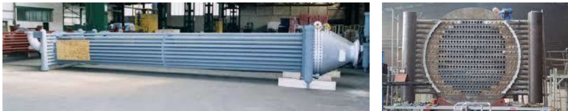
Figure 3.7: (a) Syngas cooler. The smaller cylinders perpendicular to the pipes are for inlet and outlet of the cooling medium. (b) Top view of a syngas cooler. It shows the large number of pipes, present to create a large contact surface with the cooling medium are visible (Weidenfeller et al., 2016)
