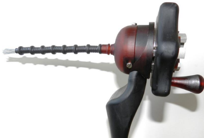
Figure 4: Friction based transport mechanism by de Kater [4].
