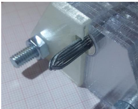
Figure 26: Two pairs of two soldered wire ropes with bent tips opposing each other. On both sides to prevent tissue from falling out four straight wire ropes are placed.
