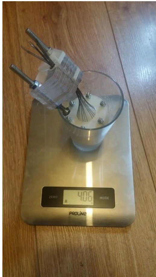
Figure 81: Measurement setup for measuring friction force of four magnets.
