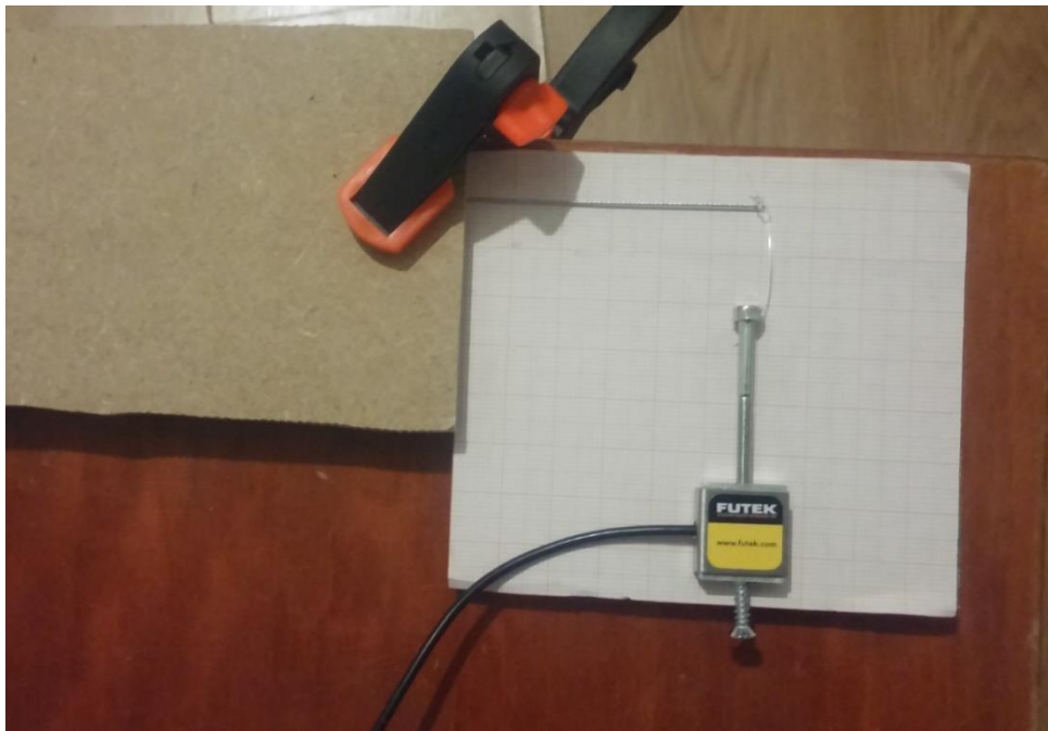
Figure 63: Bending test setup. A Futek force transducer connected to the wire rope.
