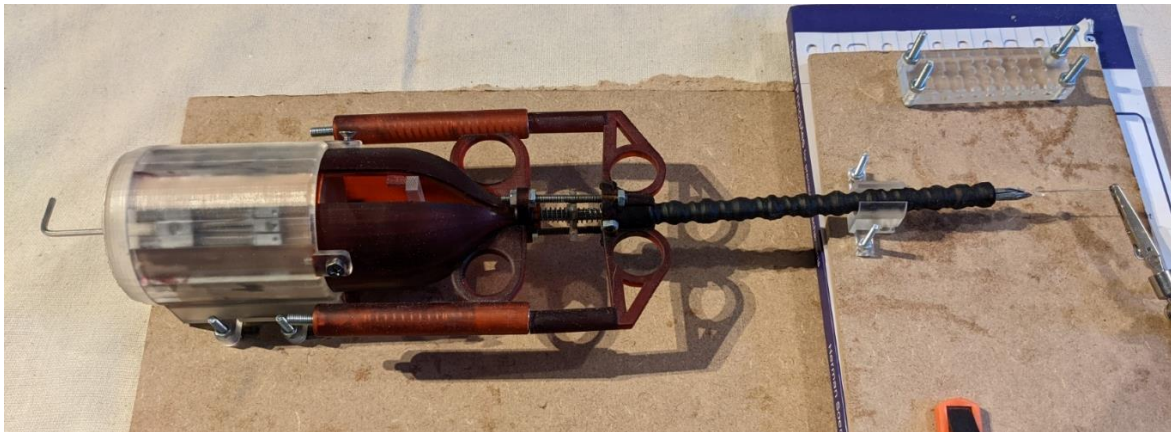
Figure 51: Test setup for grasping tissue samples. The needle is shown with a phantom tissue sample from the mould. To grasp the tissue the grasper is opened, slid forward over the sample, and closed.
