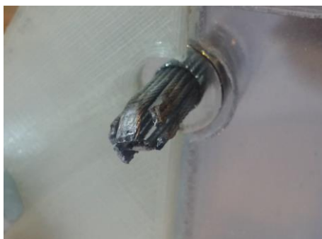
Figure 27: Two pairs of two soldered wire ropes with bent tips opposing each other. On both sides to prevent tissue from falling out two pairs of three soldered straight wire ropes are placed.
