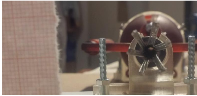
Figure 50: Setup to measure opening diameter of the grasper. Millimetre paper to use as scale is on the left.
