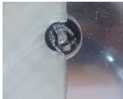
Figure 27: Two pairs of two soldered wire ropes with bent tips opposing each other. On both sides to prevent tissue from falling out two pairs of three soldered straight wire ropes are placed.
