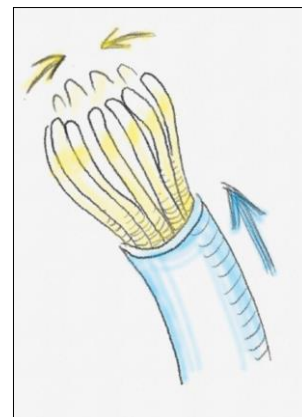
Figure 8: Proposed concept by Paul Breedveld. Displacement between the wire ropes and the sheath straightens the wire ropes and closes the grasp.
