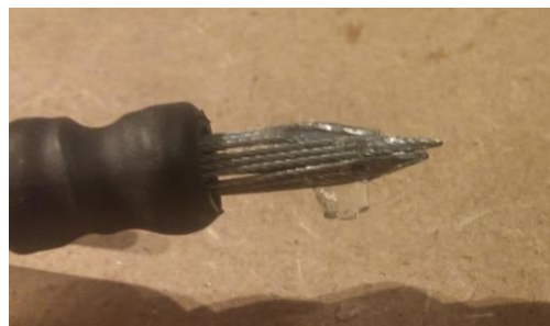
Figure 52: Cylindrical tissue being constrained by friction of two wire rope pairs.
