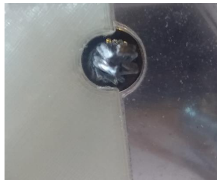
Figure 26: Two pairs of two soldered wire ropes with bent tips opposing each other. On both sides to prevent tissue from falling out four straight wire ropes are placed.
