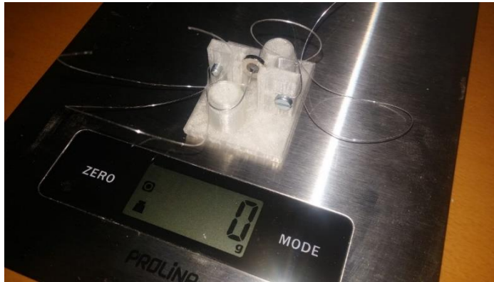
Figure 69: Measurement of detachment force threshold between magnet and wire rope.
