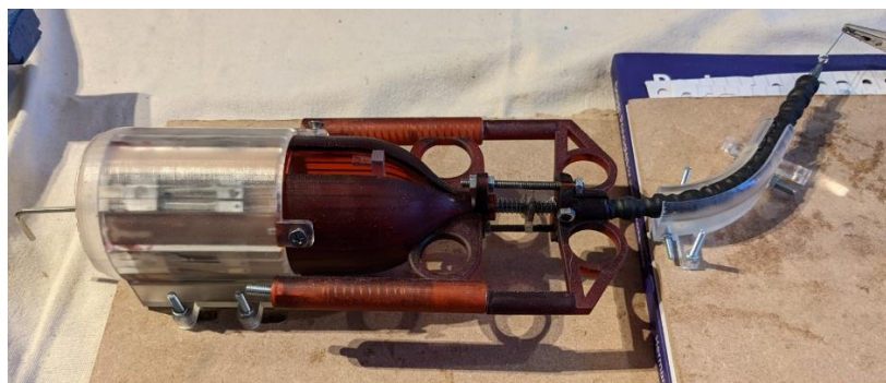
Figure 57: Test setup with bent configuration. The bend displayed has a radius of 59mm and an angle of 60 degrees.
