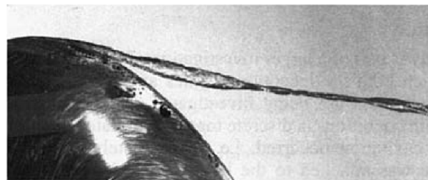
Figure 2.5: High-speed photograph of tip vortex cavitation (Maines and Arndt, 1997a).
