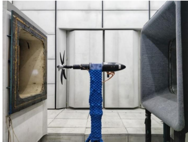
Figure 6 – Propeller performance test in D5 acoustic wind tunnel.
