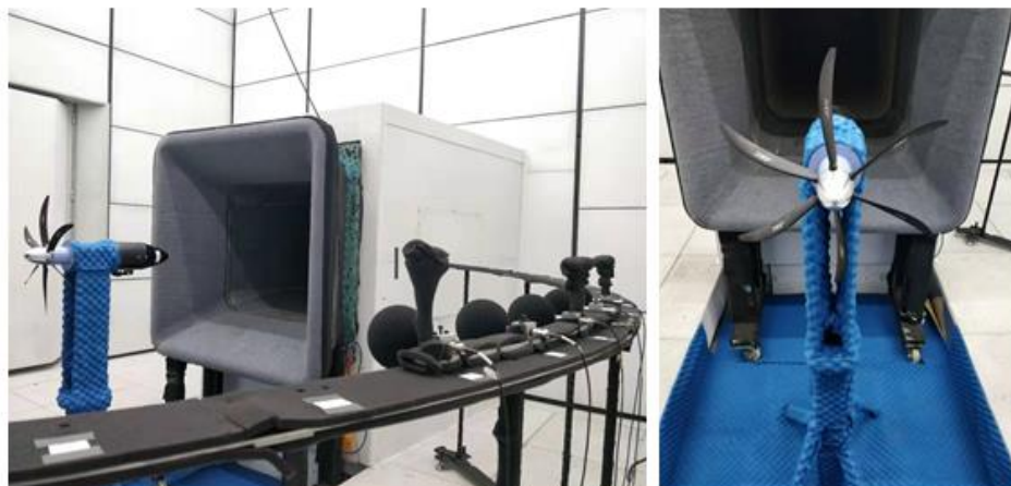
Figure 7 – The acoustic measurement setup for the test model propeller.
