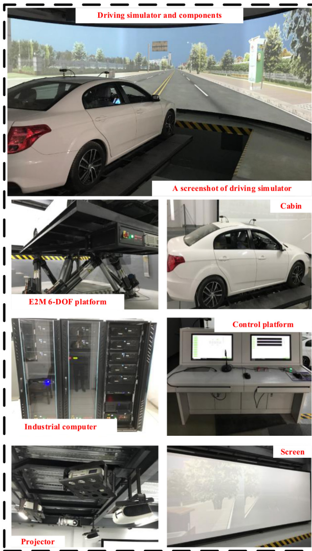
Fig. 4. Driving simulator and components.
