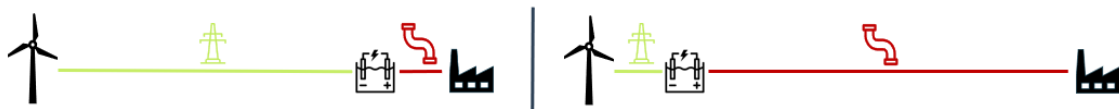
Figure 5.2: A simplified schematic illustration of two different locations for electrolyzers. The left picture shows an electrolyser located nearby hydrogen consumption with, as a result, a larger dependence on an electricity grid for the transport of offshore wind energy. The right picture shows an electrolyser located nearby renewable energy production with, as a result, a larger dependence on a gas grid for the transport of offshore wind energy.
