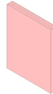
Structural timber frame partition wall panel (2400x308x3000mm)
