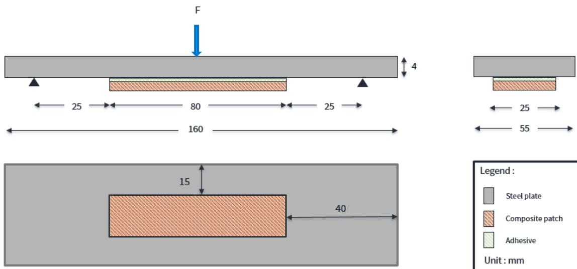
**Figure 1.** Schematic of a composite-strengthened steel plate.
