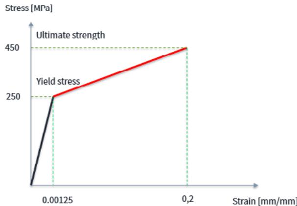
**Figure 2.** Stress-Strain bilinear law for A36 Steel.
