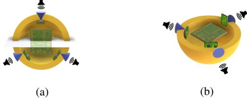
Fig. 3: Orientation of the sensor node with (a) 1 mic above mid-plane (worst case) and (b) 3 mics in mid plane (best case).
