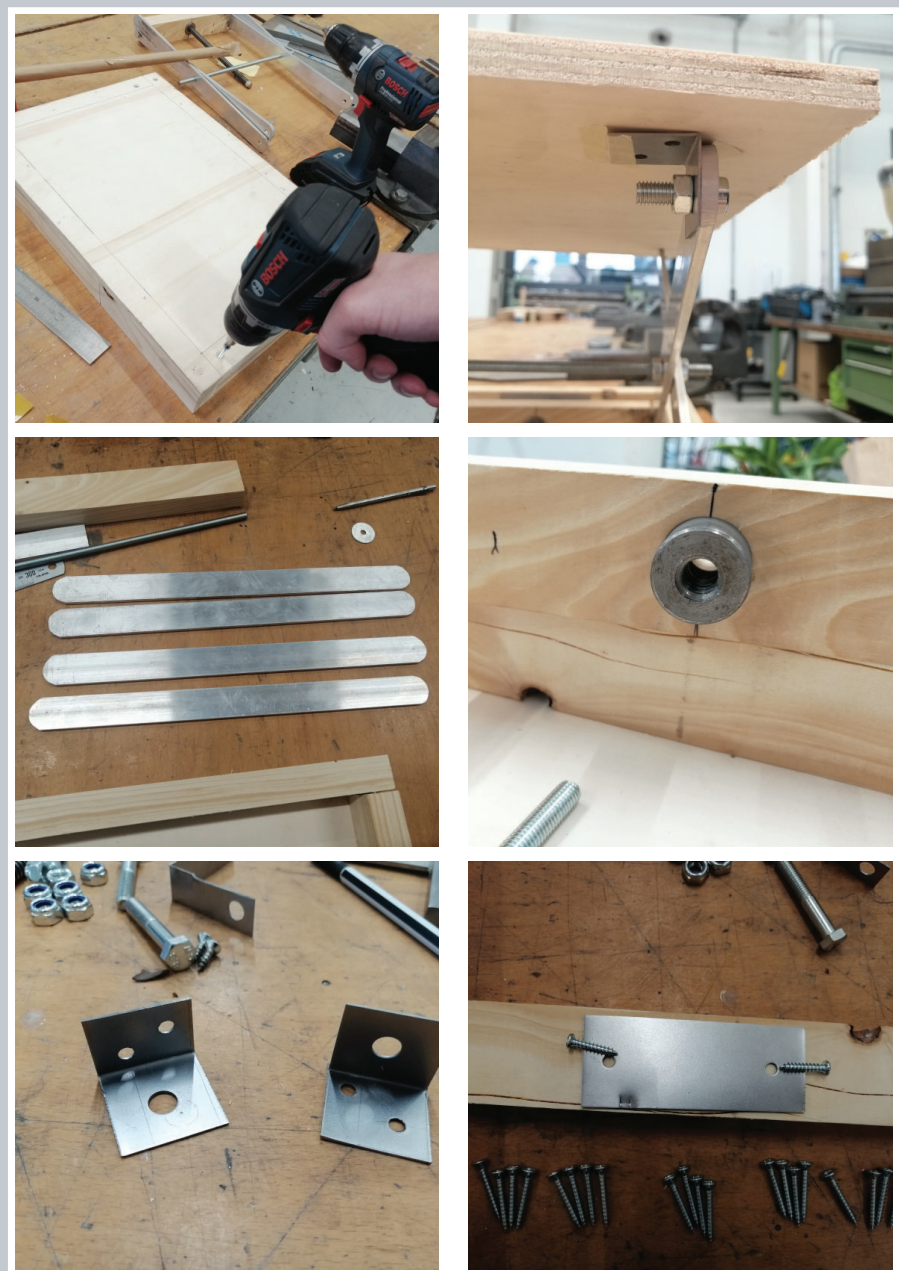
Image 8.1. Collage of scissor frame assembly.
