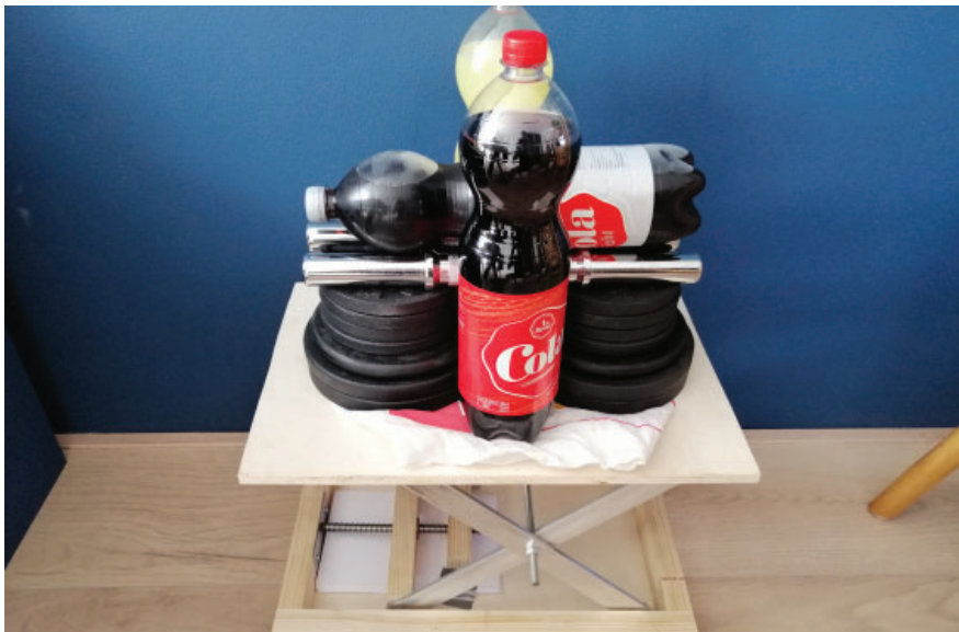
Image 8.5. Spindle handles 30 Kg downward force.
