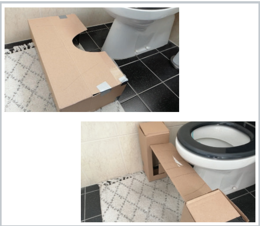
Image 5.1.A & 5.1.B Cardboard prototypes of footstool.
