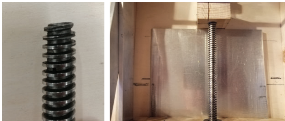
Image 8.10 Spindle angled cut-off. Image 8.11. Compensation height difference.
