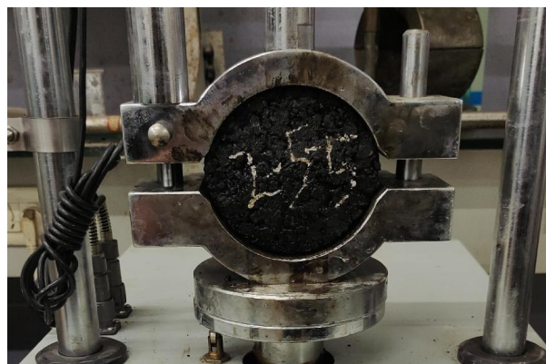
Figure 4. The standard Marshall samples under testing.
