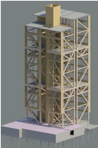
Figure 2.9: Braced frame system Treet [76]
