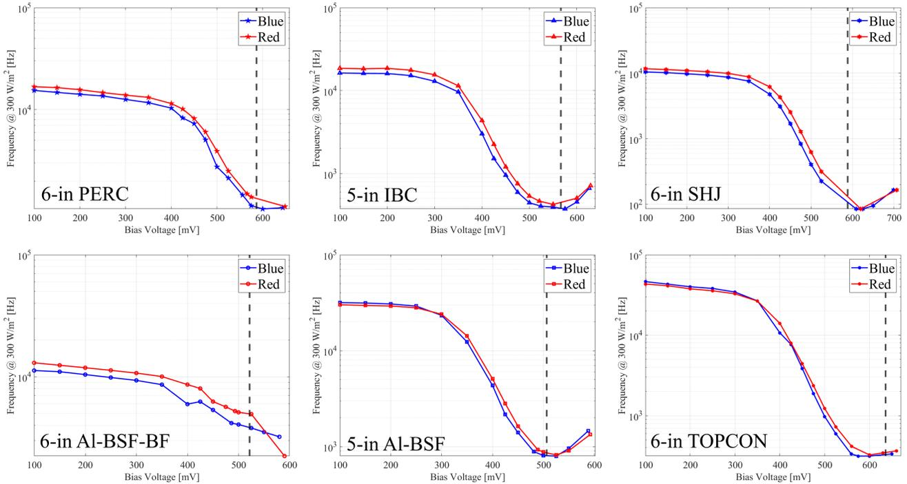
Fig. 6. Current bandwidth of the VLC system with various solar laminates under two different LED colors (red and blue) from 100 mV to open circuit condition. The dashed line indicates the  $V_{mpp}$  at STC of each solar laminate.
