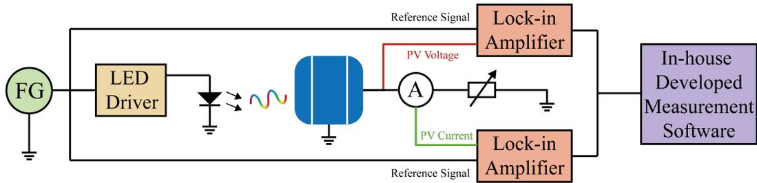
Fig. 1. Diagram of the experimental setup for bandwidth measurement of different c-Si PV architectures under colored LEDs. FG stands for function generator. The bias circuit is represented by a variable resistor for simplification. This bias circuit sets the operating point of the solar laminate and imposes a resistive load  $R_L$  in the AC circuit system.
