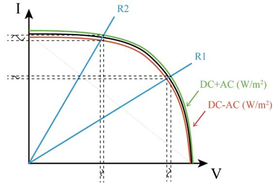
Fig. 3. Schematic representation of the response of the solar laminate upon receiving a modulated LED light signal.  $R1$  and  $R2$  represent two different load resistances. The  $I$ - $V$  curve of the solar laminate changes marginally, which creates a new set of interactions for voltage and current.
