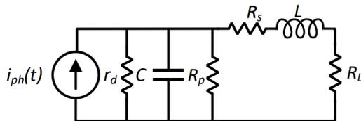
Fig. 2. Small-signal equivalent circuit model of a solar cell connected to a resistive load.
