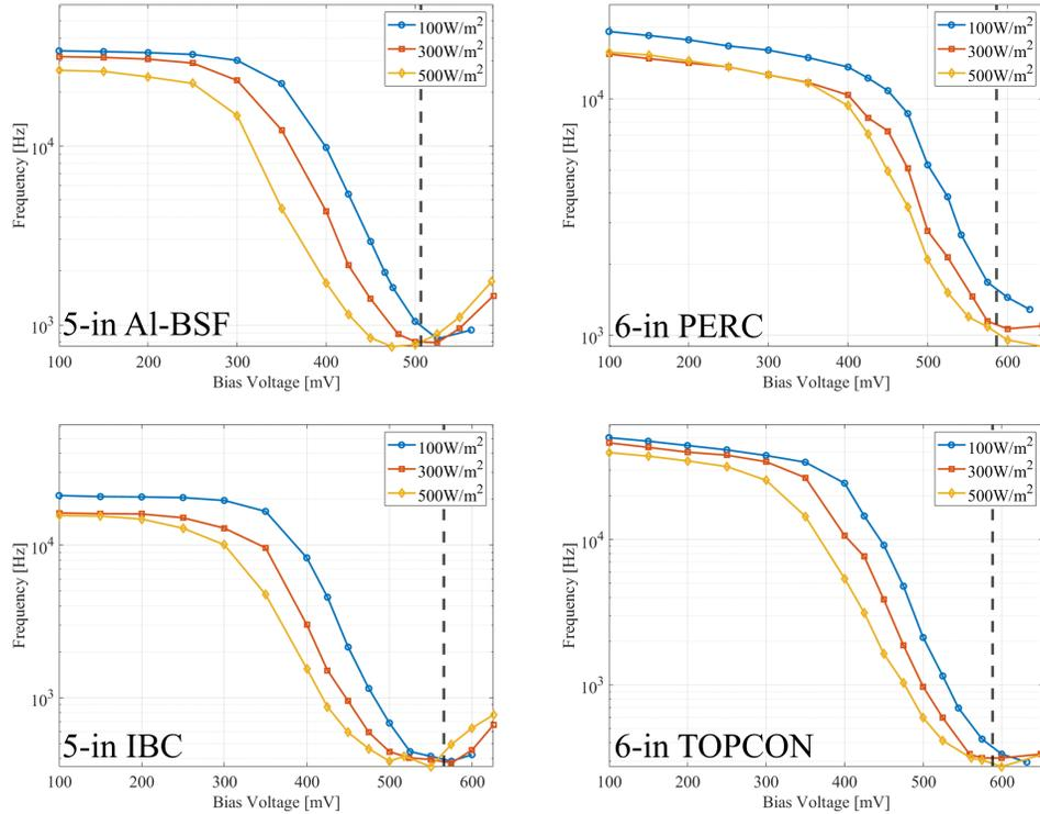
Fig. 5. Current bandwidth of the VLC system with 4 solar laminates versus different bias voltages at 3 irradiance levels of blue LED. The dashed line indicates the  $V_{\text{mpp}}$  at STC of each solar laminate.
