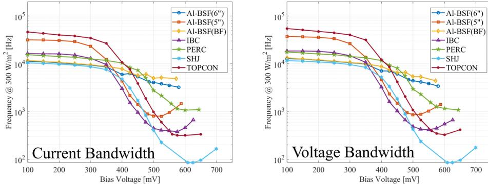
Fig. 4. Current and voltage bandwidth of the VLC system with different c-Si PV architectures at various bias voltages under  $300 \text{ W/m}^2$  blue LED.
