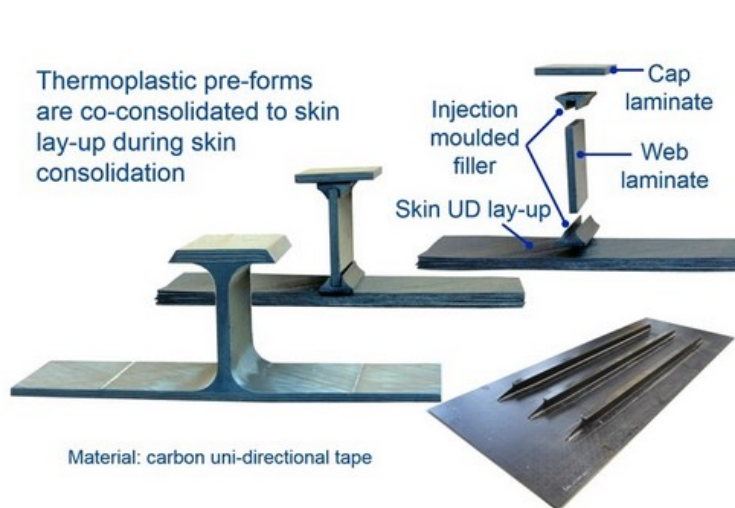
Figure 3.7: Butt-joint technology using injection moulded fillers 14
