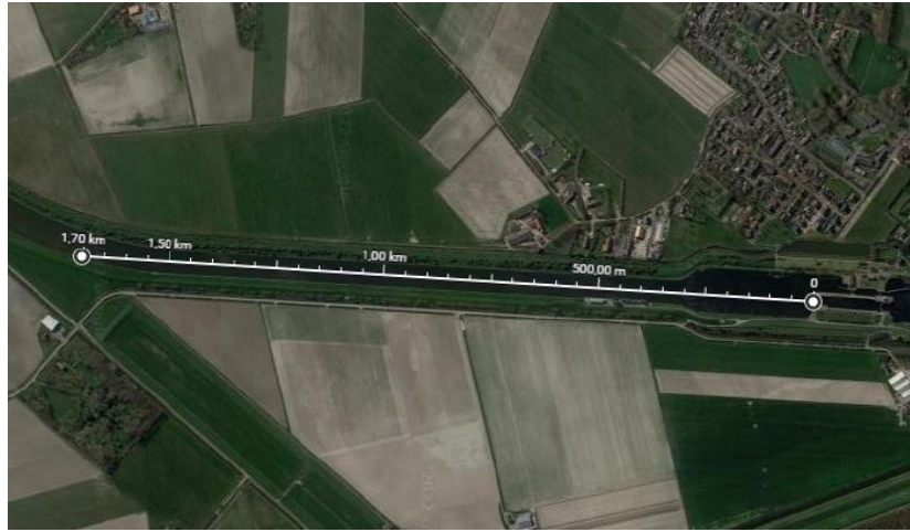
Figure E.3: The distance over which a wave can be built up in the canal [11]
