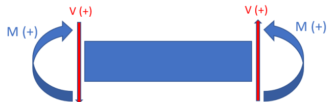
Figure 8.6: Sign Convention for positive bending moment and shear forces
