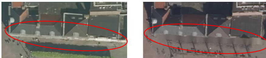
Figure 2.2: Ortho-Image (left) and trueortho-image (right) of same scene at different time steps
