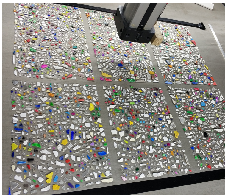
Figure 3. Near-Infrared (NIR) scanning of plastic flakes samples from waste to build databases. Each particular plastic formulation have a distinct fingerprint with its NIR spectral features which can allow, if carefully processed, for an extremely fine and specific sorting.
