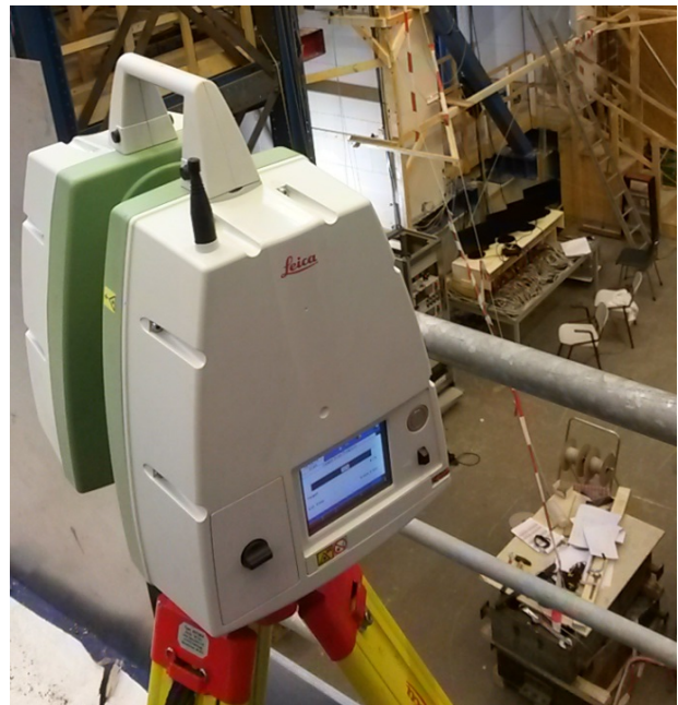
Figure 2. Leica ScanStation C10 used during field data collection.
