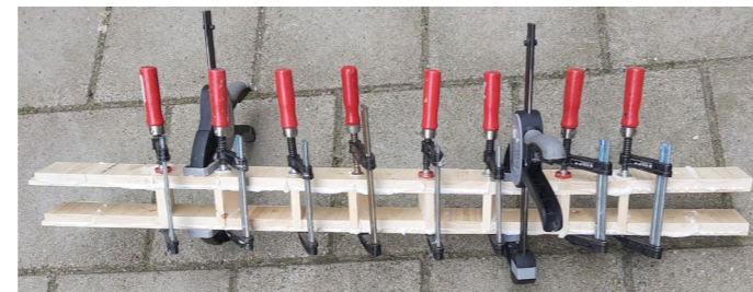
Figure 74: Direct assembly of boxfloor element
