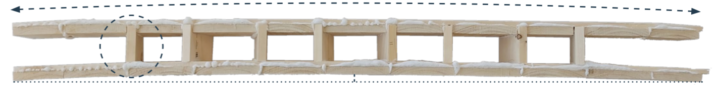
Figure 75: First curved boxfloor element with self-shaping principle.
