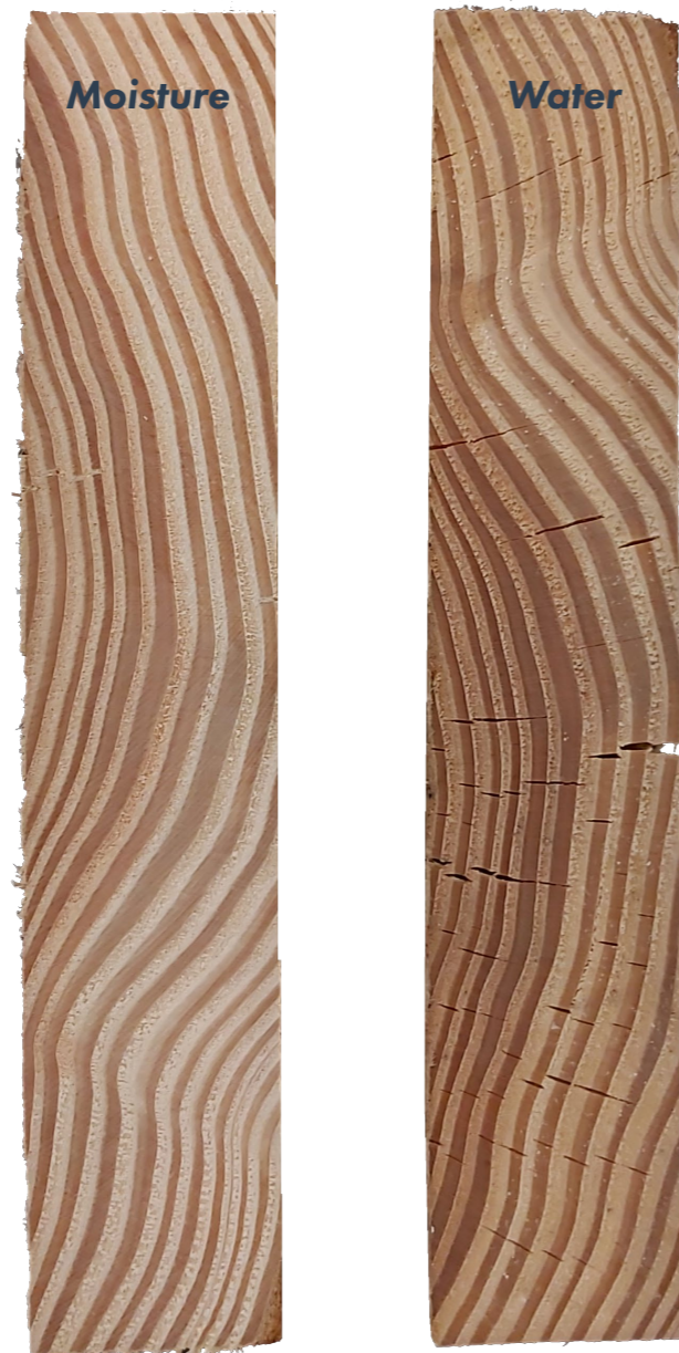
Figure 65: Crack forming due to water treatment
