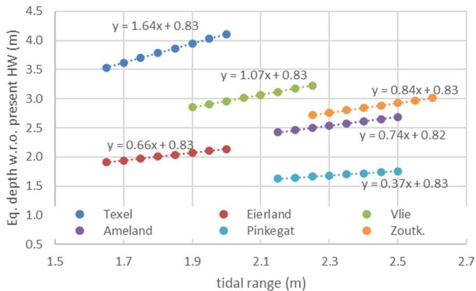
**Fig. 6** Relation between tidal range and equilibrium water depth for the various tidal basins in the Dutch Wadden Sea, derived from the analysis based on a linear relation between equilibrium volume and tidal prism. For each basin the most left point represents the initial state with the tidal range used in previous applications of ASMITA to the Wadden Sea inlets, and the coefficient in the linear relation is such that the equilibrium depth at this initial state remains the same as in Fig. 4
