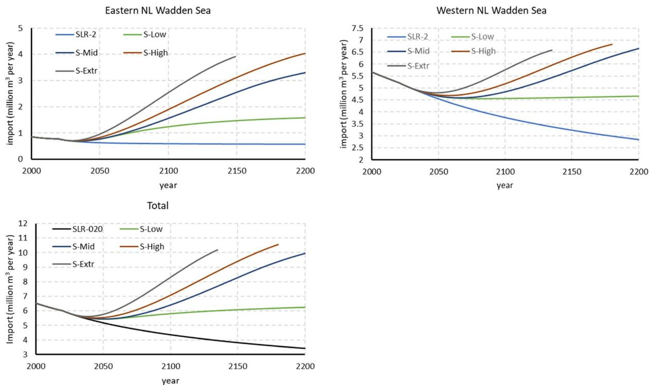
**Fig. 10** Simulated sediment import to the eastern part (Zoutkamperlaag, Pinkegat and Ameland Inlet), western part (Vlie, Eierlandsegat and Texel Inlet) and the whole Dutch Wadden Sea
