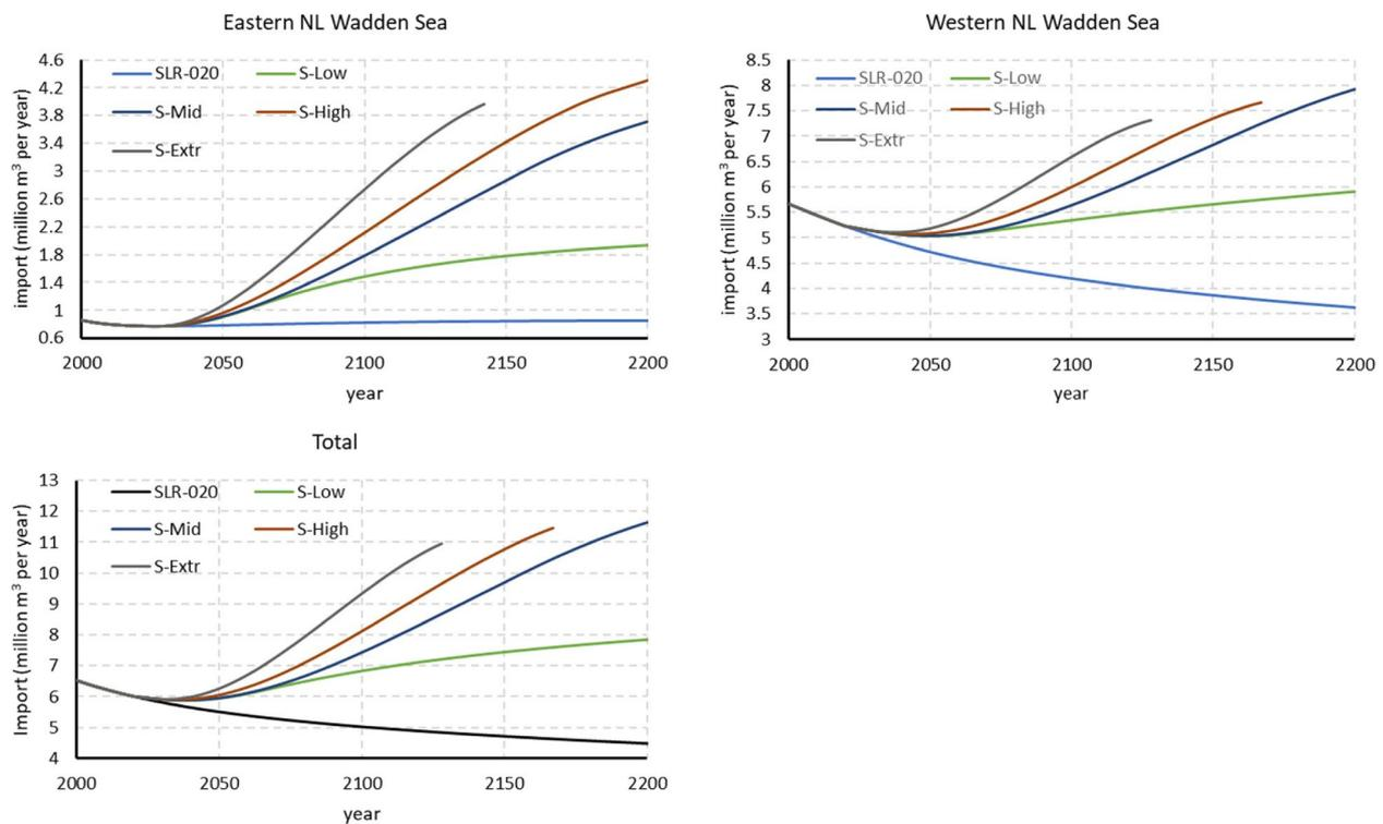
**Fig. 8** Simulated sediment transport rate to the Eastern part (Zoutkamperlaag, Pinkegat Z and Amelanderzeegat), the western part (Vlie, Eierlandsegat and Texel Inlet) and the whole Dutch Wadden Sea for the various SLR scenarios. Note that after drowning in a basin the sediment transport rate through the inlet is kept constant to make this figure
