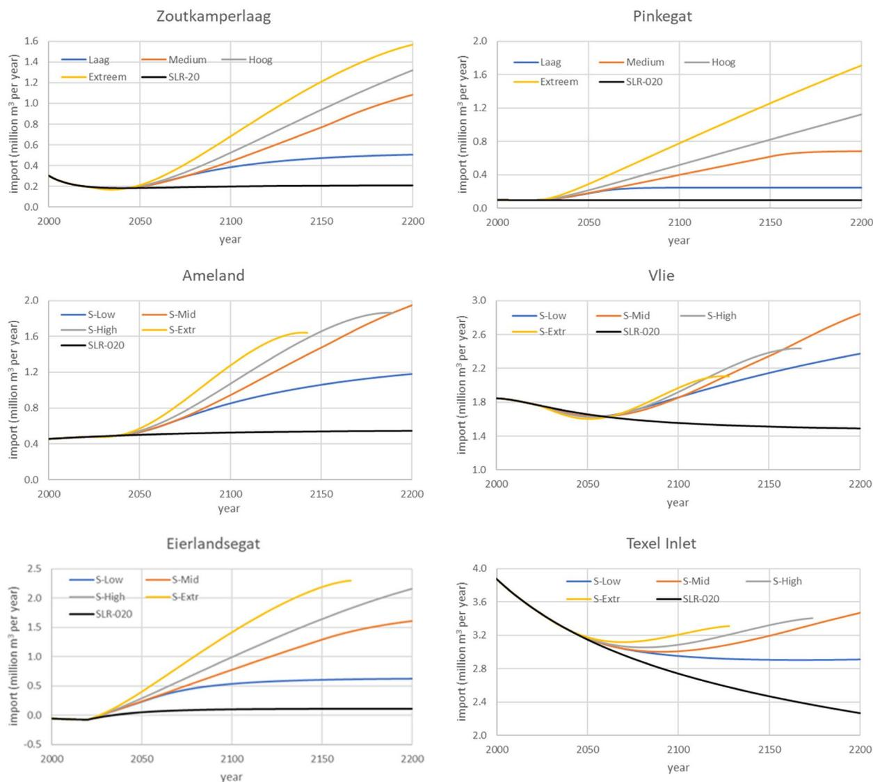
**Fig. 7** Simulated sediment transport to the Wadden Sea through the various tidal inlets for the SLR scenarios considered. Note that SLR-020 represents the case without change in the ongoing SLR rate in the last century (i.e., a constant rate of 2 mm/y). Note that series which stop before the end of the simulation period indicate drowning of the tidal flat under that scenario
