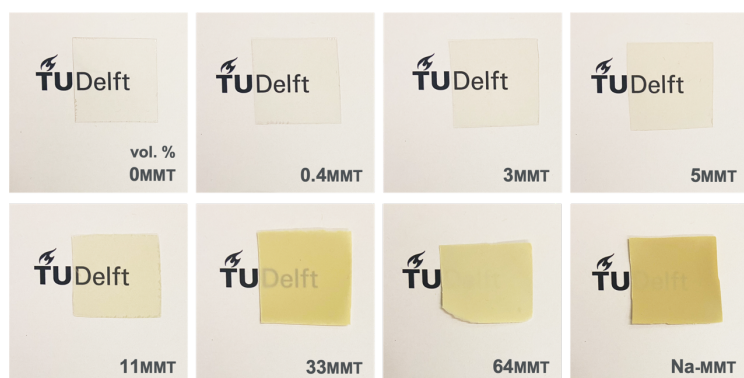
Figure S4.5. Images of gelatin/MMT nanocomposite films. The film thickness was around 0.2 mm. The notation XMMT classifies the composite film in terms of the determined MMT volume fraction ( X\% ), on a gelatin/MMT basis.
