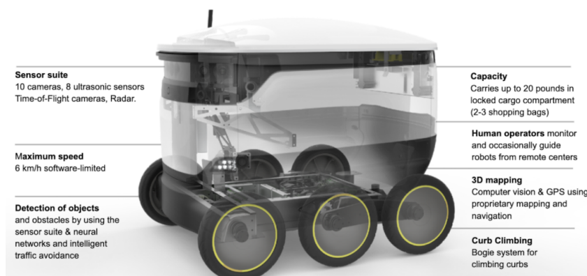
Figure 3.1: Specifications of Starship's delivery robot (Cooper, 2021).
