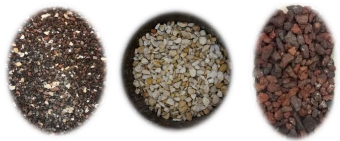
Fig. 18. The three types of nodules used in the experiments; red nodules (left), white nodules (middle) and lava nodules (right).
