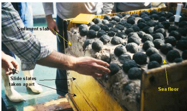
Fig. 1. Undisturbed nodule-sediment sample illustrating the burial of nodules (Museum National d'Histoire Naturelle Box Corer [19]).
