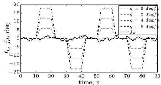
Fig. 5. Target and disturbance forcing function time traces.
