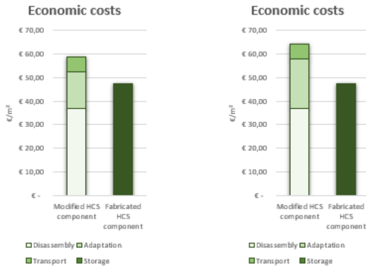
Figure 63. The economic costs per m2 for scenario 2 [Right: single-family house; Left: low-rise apartment building].
