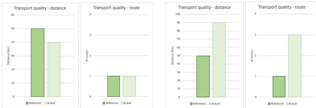
Figure 52. The 'sensitivity' of the additional performance related to the transportation process [Left: the transportation performance are lower than the reference situation – the impact is low; Right: the transportation performance are higher than the reference situation – the impact is high and the reuse potential factor will be lower].
