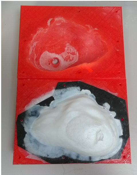
Figure E.2: Solid state liver model is acquired after a 40 hours freezing period.
