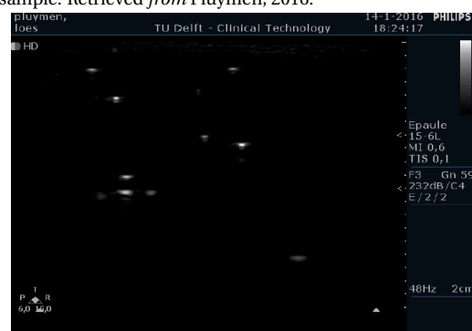
Figure 2.16: Ultrasound visual reconstruction of 100% plasticizer PVC sample. Retrieved from Pluymen, 2016.
