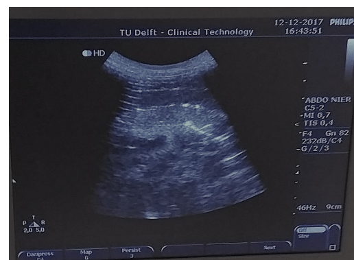
Figure 6.22: Ultrasound image reconstruction of the integrated liver model taken from intercostal probe position.
