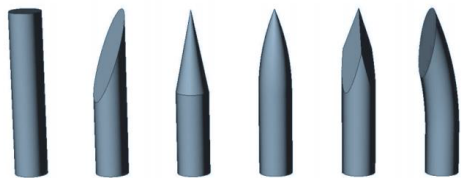
Figure 2.7: Common needle tip shapes, left to right: blunt, beveled, conical, sprotte, diamond, Tuohy. Adopted from van Gerwen et al., 2012.
