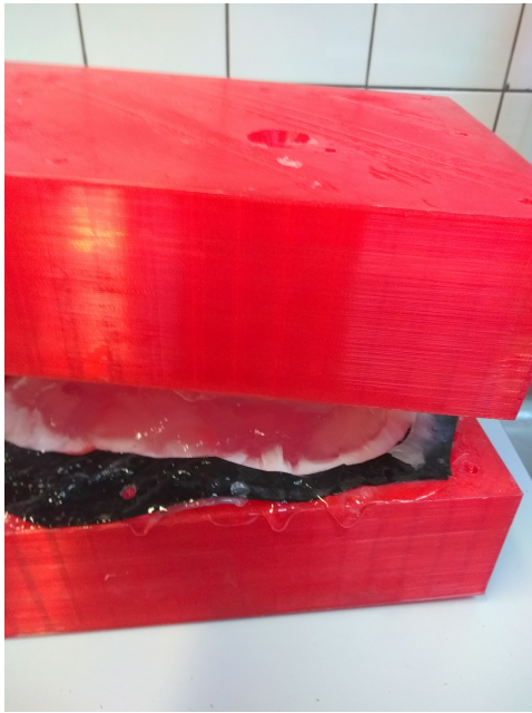
Figure E.1: Non-solid state of the liver model after a 16 hour freezing period.
