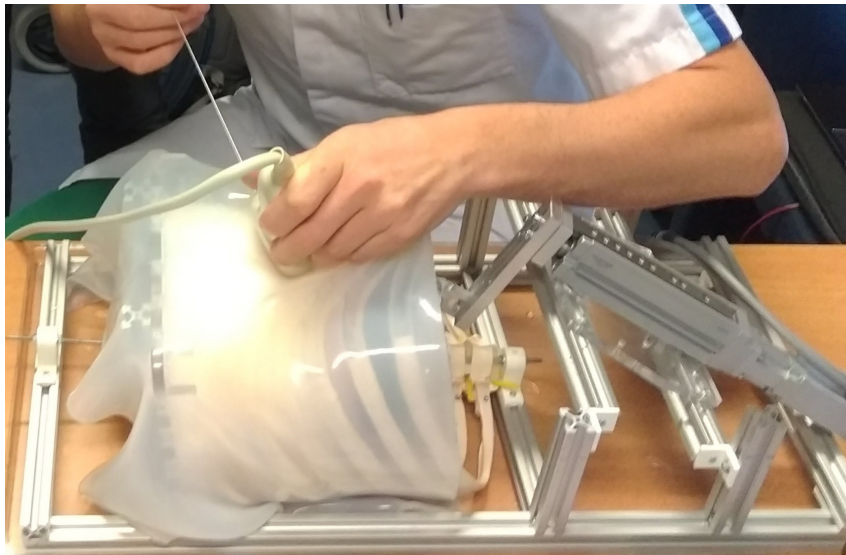
Figure 6.1: Evaluation of the phantom during needle insertion under ultrasound guidance.
