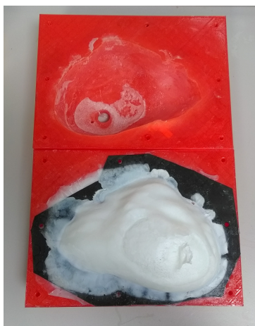
Figure 4.8: Pour-molding of the liver in 3D printed mold.
