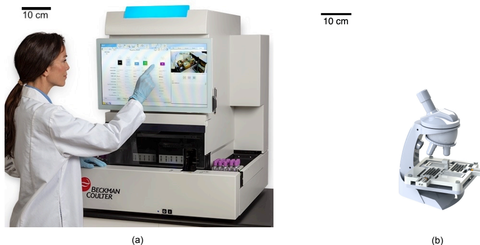
Figure 4.22: (a) A standard hematology analyzer that is used for blood smear analysis [8]. (b) The compact stage that was designed as alternative to a hematology analyzer. Note that it is shown without a power source, microcontroller, driver or computer.
