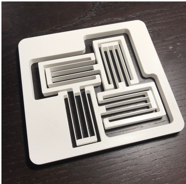
Figure 5.1: First prototype 3D-printed out of PLA for proof of concept.
