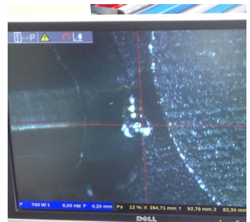
Figure 12: Connection of tube head (left) and nozzle head (right)
