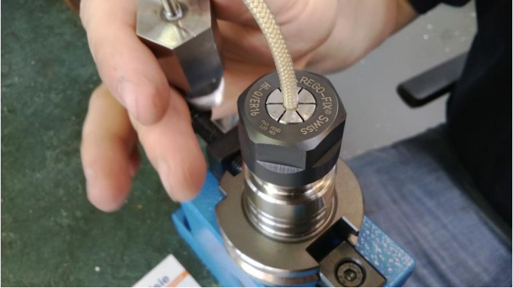
Figure 30: Tube head fixated in lathe
