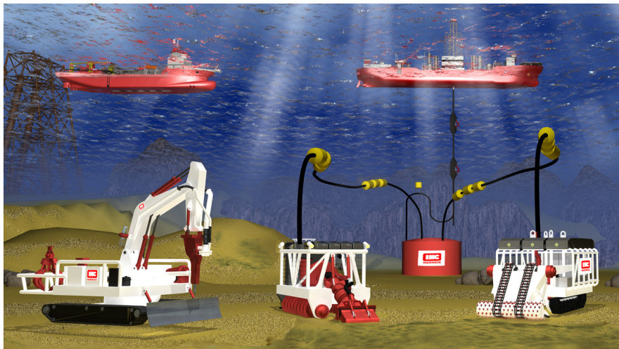
Figure 1-1: An artist impression of deep sea mining equipment operating at the sea bed. This equipment has to be lowered carefully to the sea bed using lifting operations. Image courtesy of IHC
