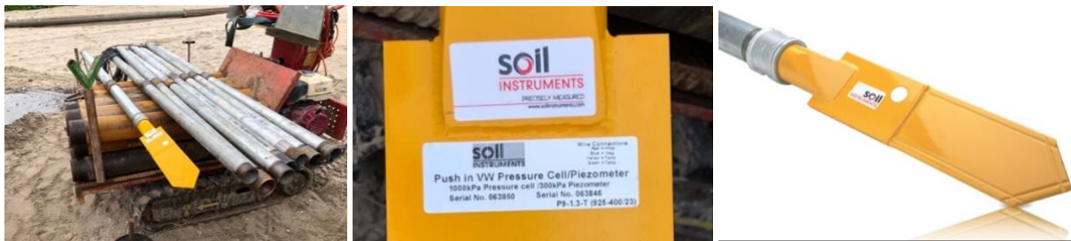
Figure 2.10: Left: Spade cell RijnlandRoute (Verloop, 2019). Middle: Spade cell information RijnlandRoute (Verloop, 2019). Right: Spade cell head [21]
