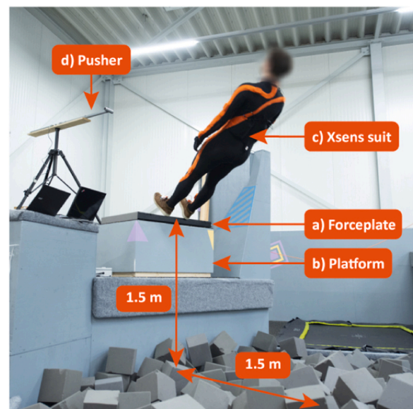
Fig. 1. A snapshot from one of the experimental trials. Participant falling from the force plate (a) that is located on the platform (b) into the foam pit. The participant wears an Xsens motion-capture suit (c). The device for pushing the participant into the pit can be seen on the left (d).
