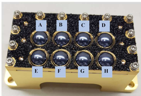
Fig. 7. a) Polar plots summarizing the final pointing error for a re-aligned 4 \times 2 pixel array using the large lenses. The pointing direction is seen as the propagation direction of light that is "emitted" from the detector at the back of a lens and transmitted through the lens towards the far-field, as seen from the reader perspective. b) Front view of the final assembled array. The front of the 8 lenses can be seen, with the 8 HEB detectors assembled on their backside (not visible).
