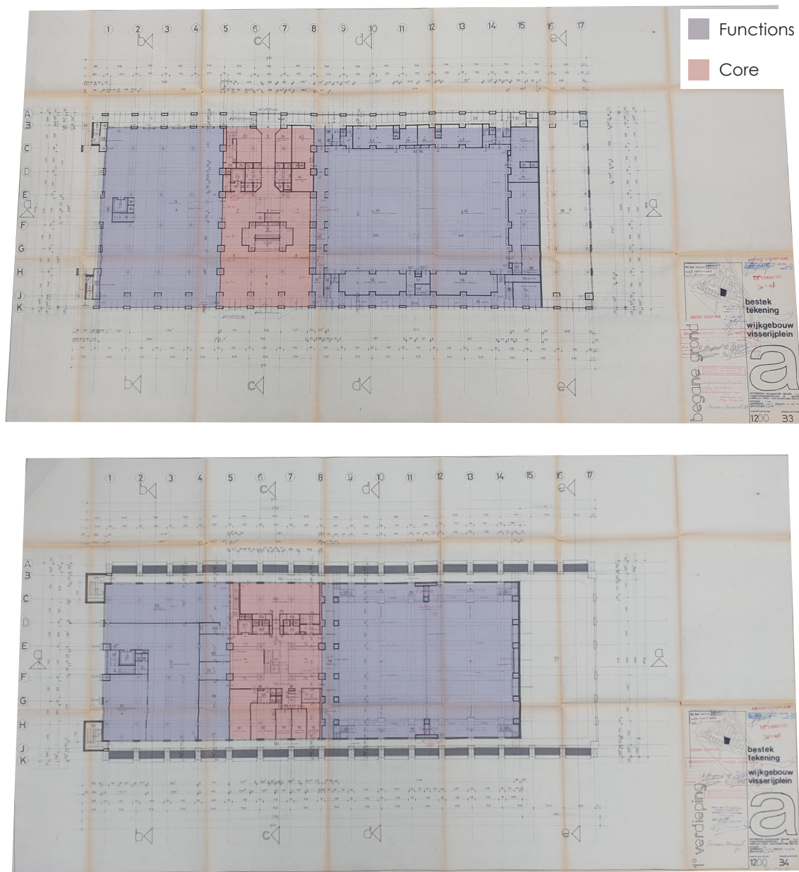
Figure 5.3. Floorplan analysis of the spaces with functions of Pier 80. Schravessande designed a core (red) and on the sides the library and multi-functional spaces (blue). (Architectencoöperatie Gouda, 1981. Stadsarchief Rotterdam).
