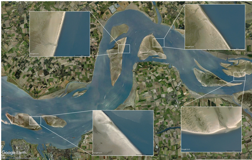
Figure 2. Google Earth satellite images showing small-scale levee formations at the channel-shoal interface in the WS. Note: Large and small images scales (bottom right) are 6 km and 200 m, respectively.
