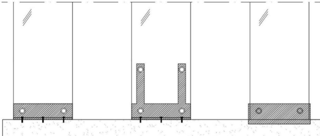
Figure 8.9: An impression of rigid shoe alternatives. It is best to use the four glass holes with a bolt. From structural alternatives, a rigid or hinged alternative should be deigned. Scale 1:20.
