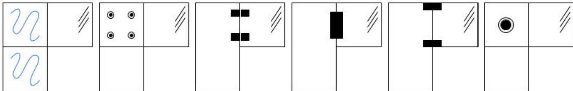
Figure 5.2: From left to right: UV-acrylic adhesive, bolted rigid, embedded connection (3x), bolted hinged.
