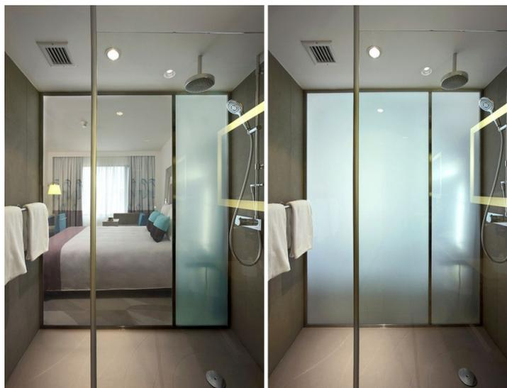
Figure 3.6: An electric current makes a glass panel translucent [12].
