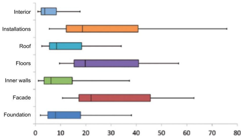
Figure 6.2: Impact of various parts on the shadow costs [37]
