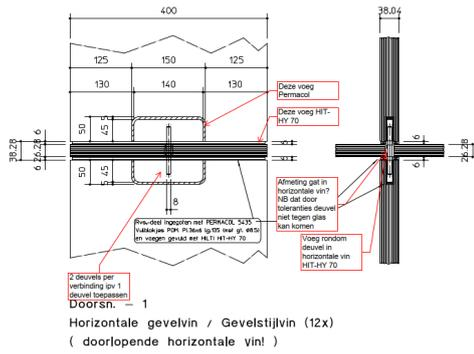
(a) A stainless-steel element is embedded in the glass fins and is covered on both sides with another glass panel. To connect the glass to the element, use is made of Permacol 5435, a 2 component PU-adhesive which serves as interlayer between the glass and glass and allows for some tolerances. The remaining gap is filled up with Hilti-HY 70, a mortar (Hybrid Urethane Methacrylate). 6x6x400 mm3 (4x)
