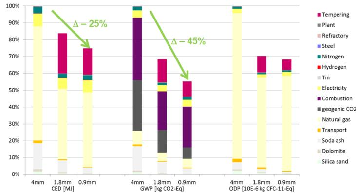
Figure 3.5: Allocation of environmental impacts: production of standard float glass (4 mm) and tempered thin glass (1.8 and 0.9 mm). Values are related to the production of a single glass pane of  $1 \text{ m}^2$ . A thinner tempered glass pane has a lower CED (Cumulated Energy Demand), GWP (Global Warming Potential) and ODP (Ozonlayer Depletion Potential). [8].
