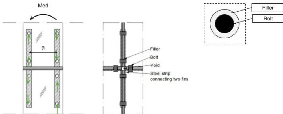
Figure I.3: Sketch of the bolted rigid connection in a straight segment.
