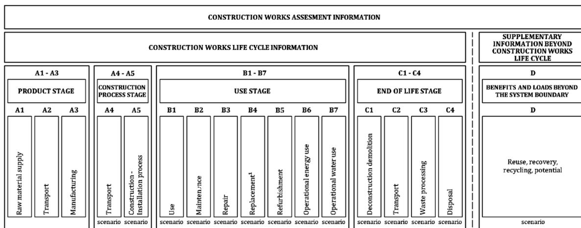
Figure 2.8: Different modules within an EPD according to standard EN 15804
