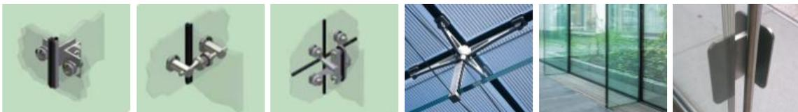
Figure 5.3: From left to right: angle spring plates [34], spider connected to a glass fin [34], fitting to a glass fin [34], point-fixed clamped [35], structural silicone adhesive [36], titanium embedded [author].
