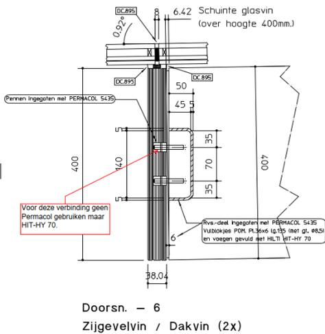
(a) similar embedded connection, only here it is used at a T-section
