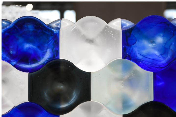
Figure 3.4: Glass waste is recycled into load bearing building applications.[11]
