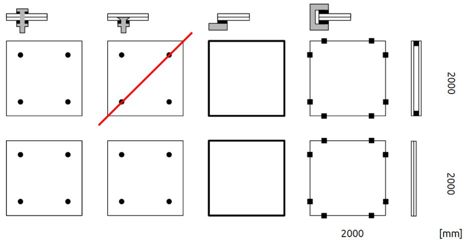
Figure 6.3: Presumed connection types. From left to right, point fitting, countersunk point fitting, structural sealant and edge clamped.
