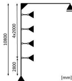
Figure 8.17: Buckling supports along the facade fin due to the perpendicular fins. The governing situation is the situation with the longest unsupported part (2.8 m). Buckling support against lateral torsional buckling in the roof beam are not shown.
