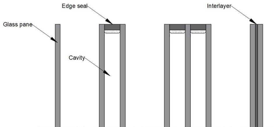
Figure 2.5: Single, double and triple glazing and a laminated glass panel.
