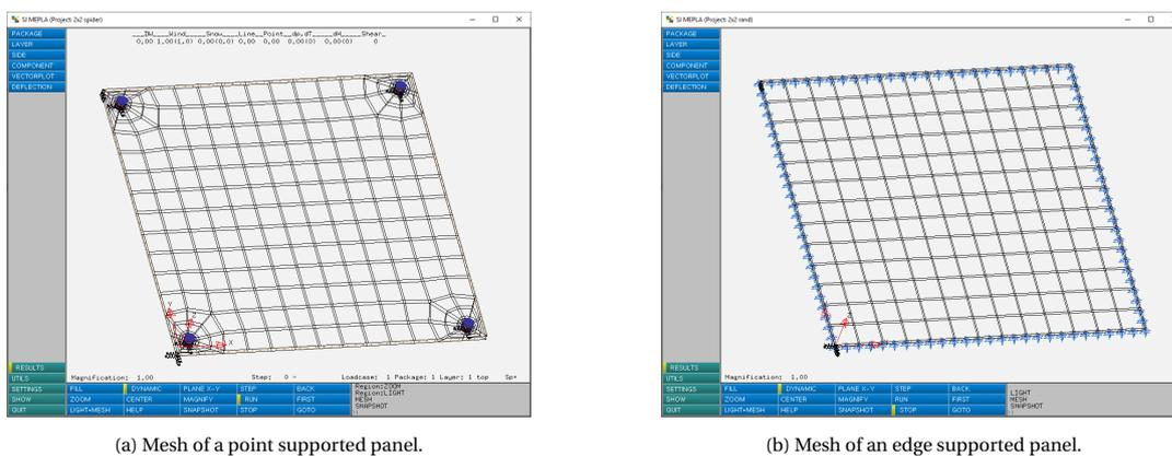
Figure H.1: Mesh size is limited by the program, but the presented mesh size is considered to be viable.
