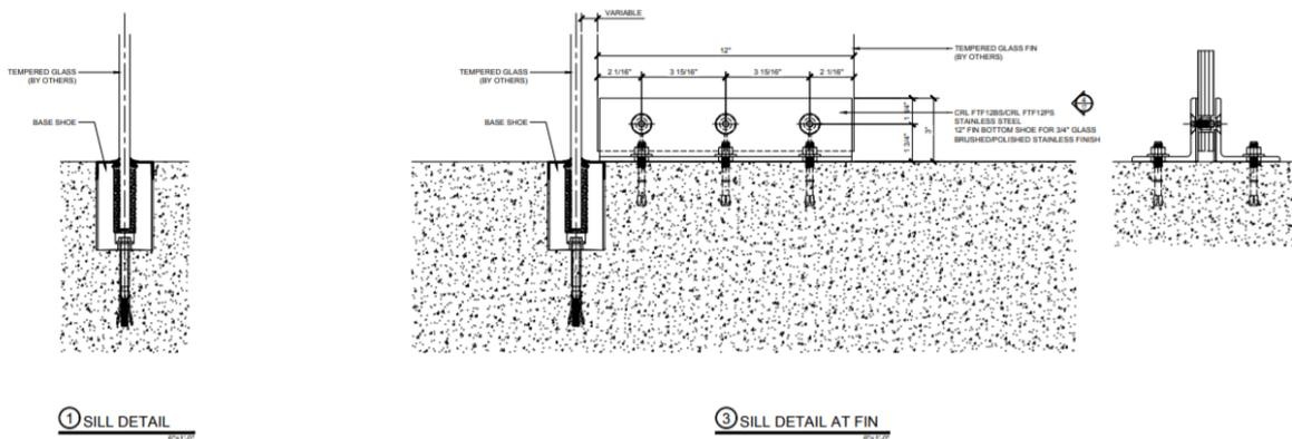
Figure 4.15: A base shoe: a mechanical connection which connects a fin to other materials. [24]
