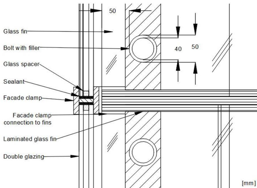
Figure 8.11: Detail of fin-facade connection. Scale 1:4.
