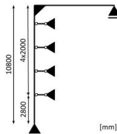
Figure I.5: The governing situation is the situation with the longest unsupported part (2.8 m).
