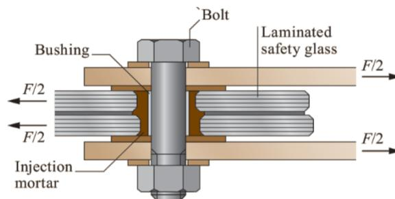
Figure 4.11: Load transfer of a point fixing in a laminated glass application. [18]
