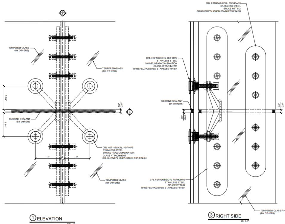
Figure 4.16: A splice fitting: a mechanical connection which connects two fins. [24]
