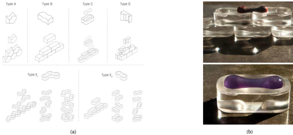
Figure 4.24: Dry stacked interlocking glass components. [29]
