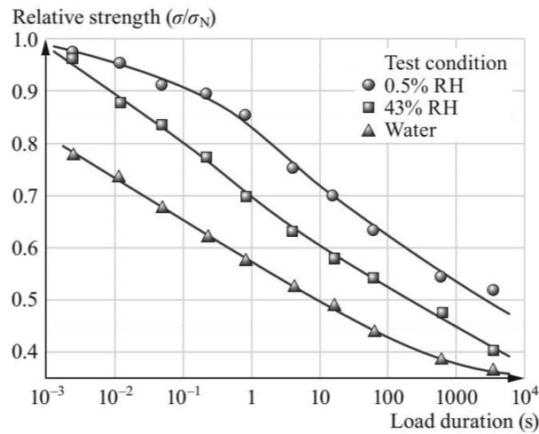
Figure 2.6: Relative strength to moisture and load duration [5].
