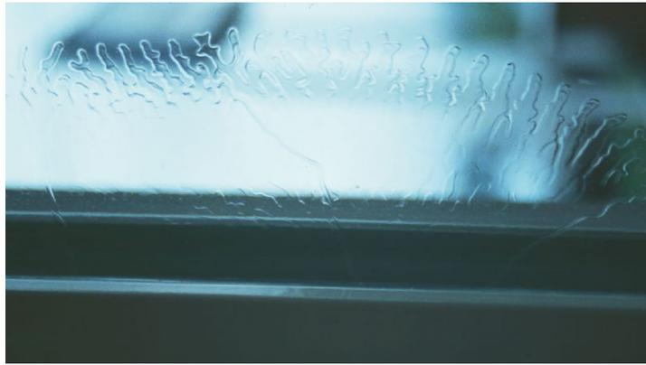
Figure 3.7: Delamination of a PVB interlayer [13].
