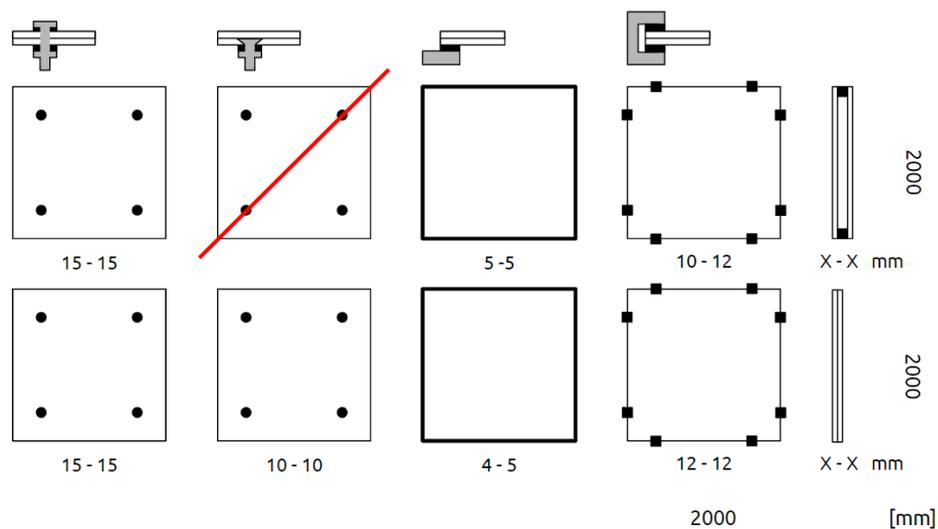
Figure 6.4: Pane thicknesses optimized to above mentioned assumptions.
