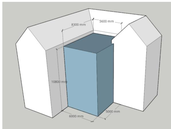
Figure 8.1: Sketch of the current design with indication of size with in white the castle.
