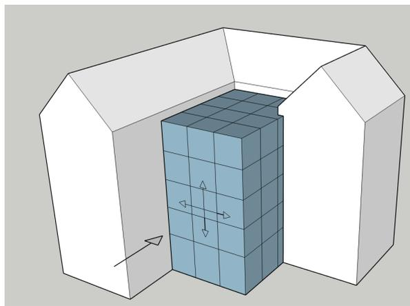
Figure 8.15: Since the moment rigid frame makes a stiff grid, the force distribution is not equal to all four sides, but dependent on the geometry.
