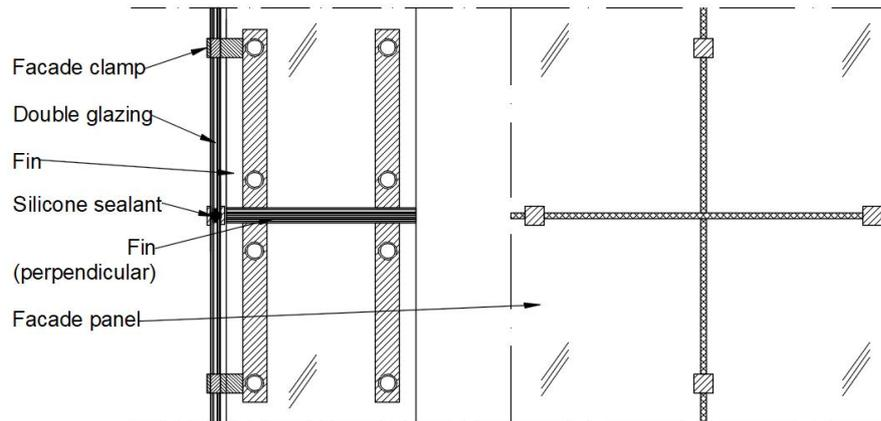
Figure 8.10: Sketch of the four point supported facade detail.
