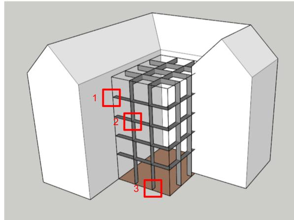
Figure 8.3: Three main types of connections for the fin. 1: fin-fin in a frame, 2: fin-fin crossing, 3: fin ending.
