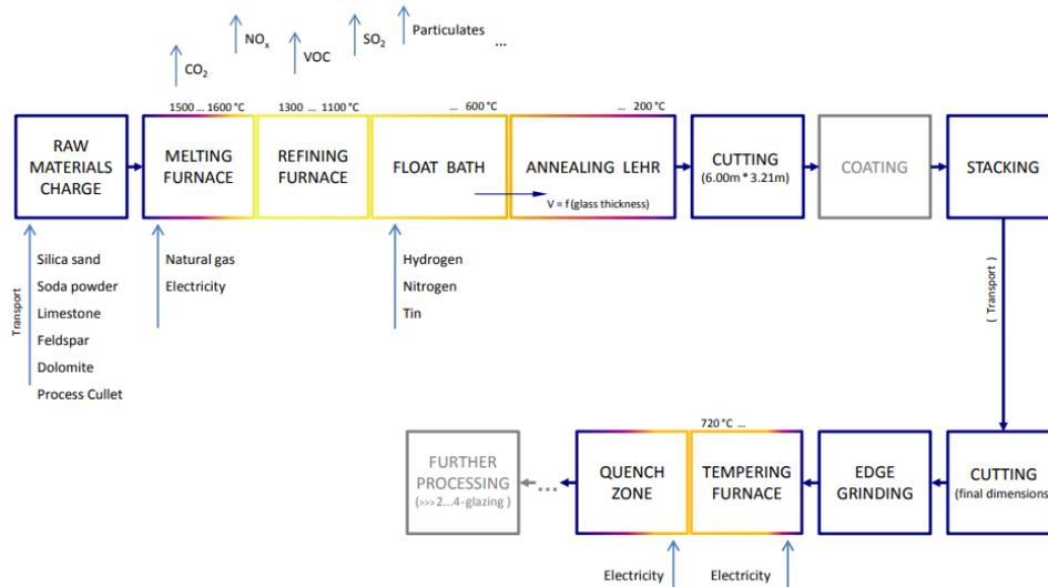
Figure 3.1: Energy processes and emission during glass production. In the top, the float glass process is shown and in the bottom, the tempering process is described. Among others, these emissions come from the production process. [8]
