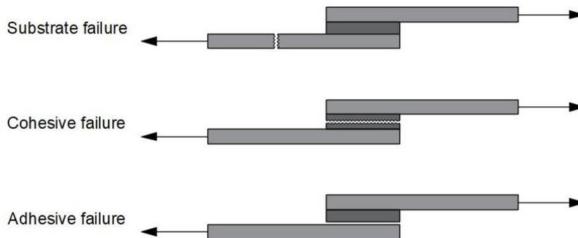
Figure 4.4: Failure mode of adhesives. An adhesive failure should be avoided.
