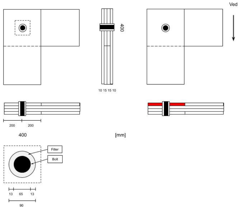
Figure D.6: Sketch of the bolted rigid connection.
