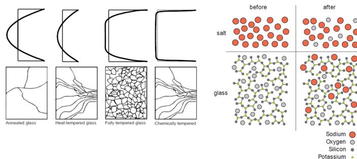
Figure 2.2: Failure pattern of different types of glass.[3]
