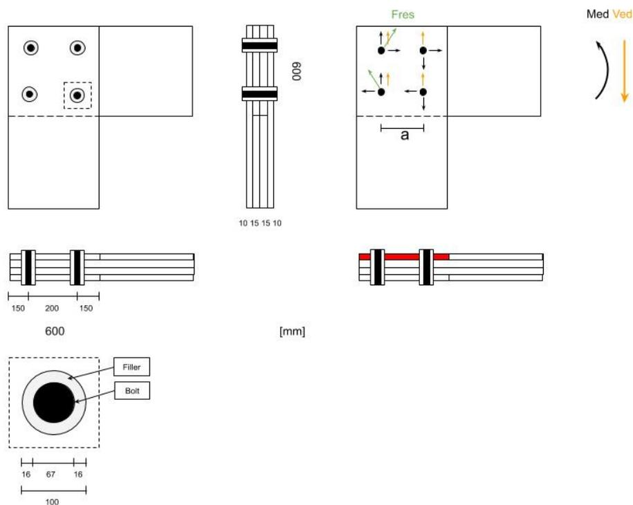
Figure D.2: Sketch of the bolted rigid connection.
