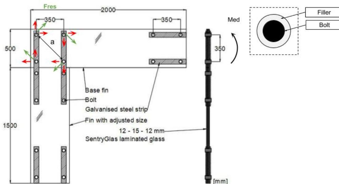
Figure I.1: Sketch of the bolted rigid connection.
