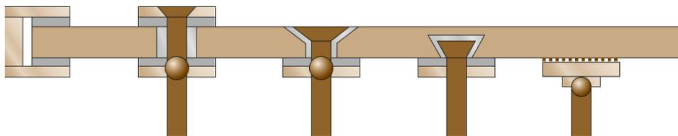
Figure 4.12: Various point fixings. From left to right, clamped on the side, a glass piercing point fixing, pierced and chamfered hole, countersunk (embedded) and adhesive based. [18]
