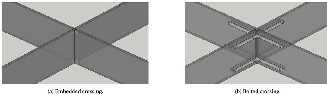
Figure 8.6: Perpendicular moment rigid crossing.
