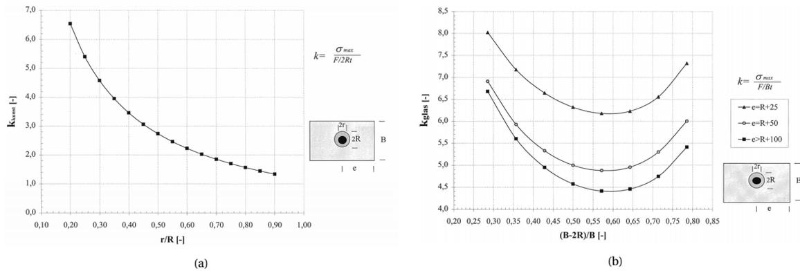
Figure I.2: Relations to derive the stresses in the glass and the filler. [38]
