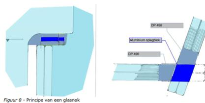
Figure B.10: Epoxy 3M DP490 is applied in the corners.
