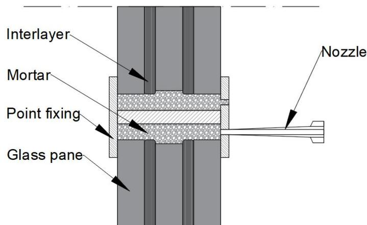
Figure 4.9: Application of a filler. Adjusted from [20].
