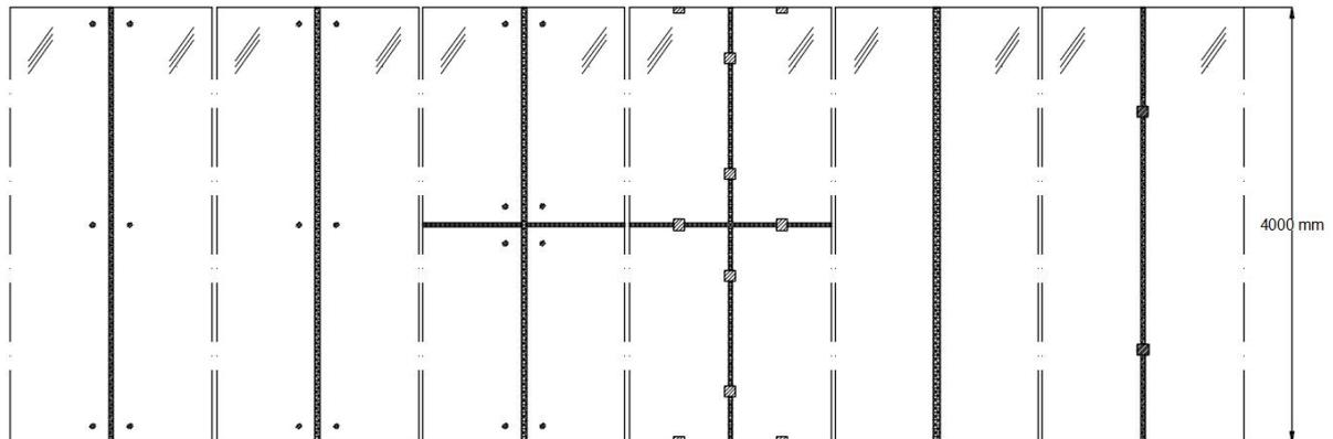
Figure 5.6: Facade connection front view. From left to right: angle spring plates, spider connected to a glass fin, fitting to a glass fin, structural silicone adhesive, point-fixed clamped, titanium embedded.
