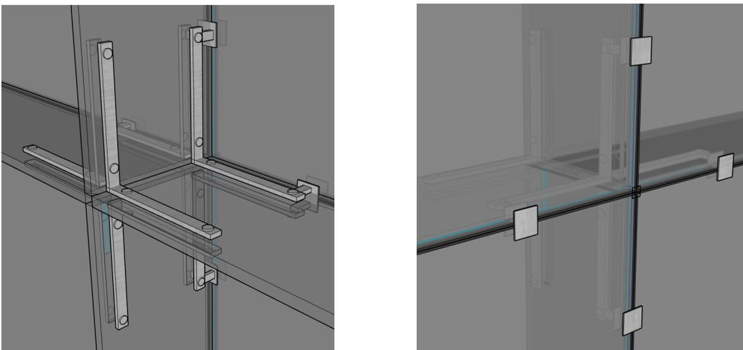
Figure 8.13: An impression of a four point spider facade clamp integrated with perpendicular connections
