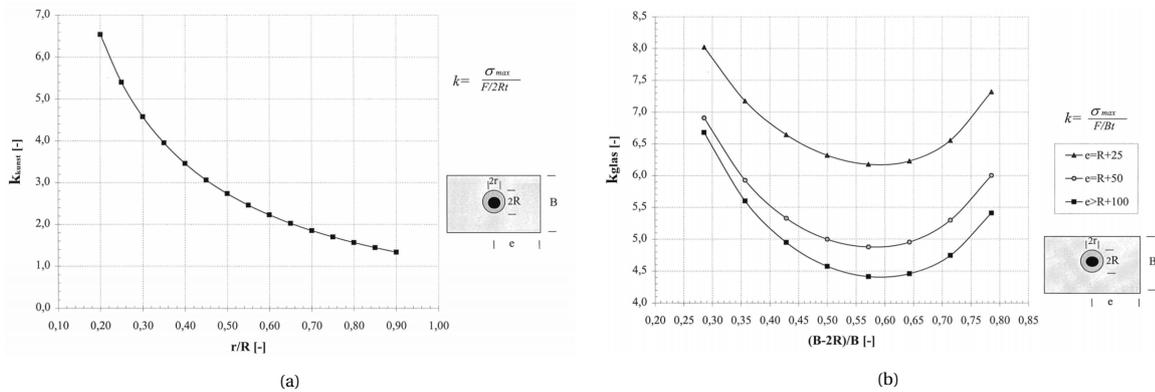
Figure I.4: Relations to derive the stresses in the glass and the filler. [38]
