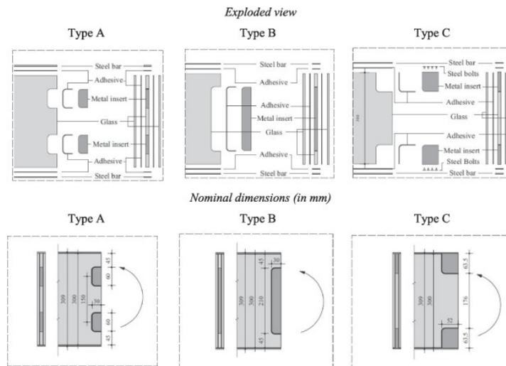
Figure D.5: Embedded connections by [39]
