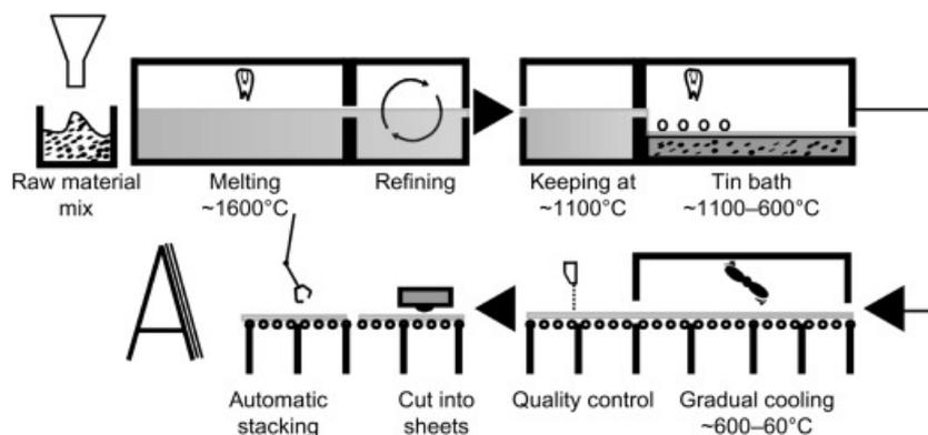
Figure 2.1: Float glass production process [2]
