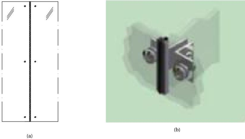
Figure E.3: Angle spring plates with point fixing to connect facade and fin.
