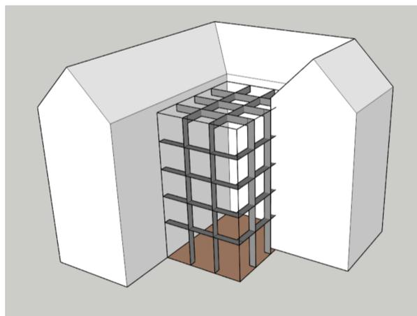
Figure 8.2: Fins are required in design for both facades and result in the roof grid.
