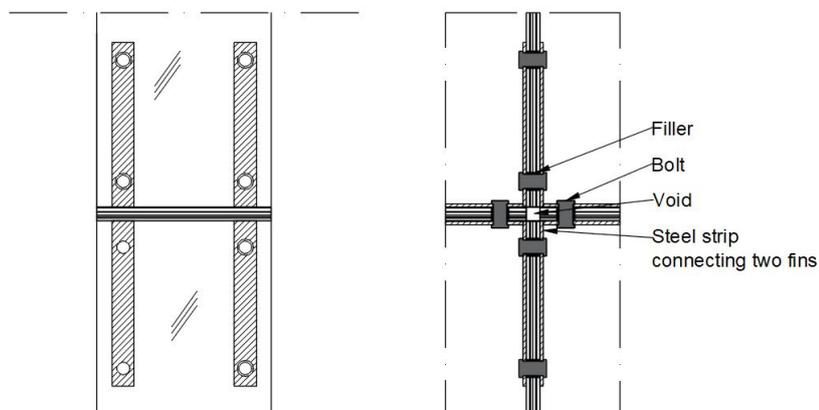
Figure 8.7: Detail of a perpendicular fin-fin crossing. Scale 1:20.
