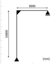
NOTE: The intermediate supports are removed in order to derive the maximum occurring situation
