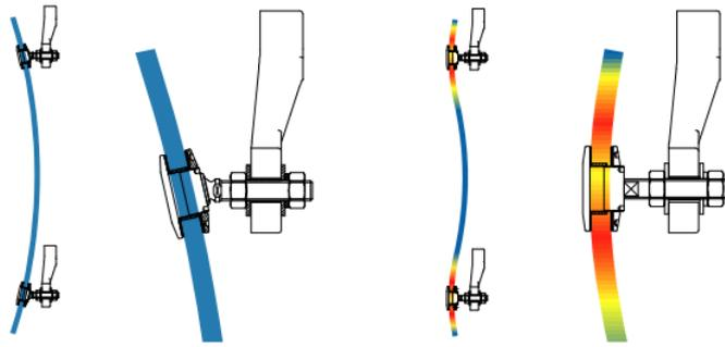
Figure 4.13: A swivel fitting decreases stresses in the glass. Red indicate higher stresses than blue. [22]
