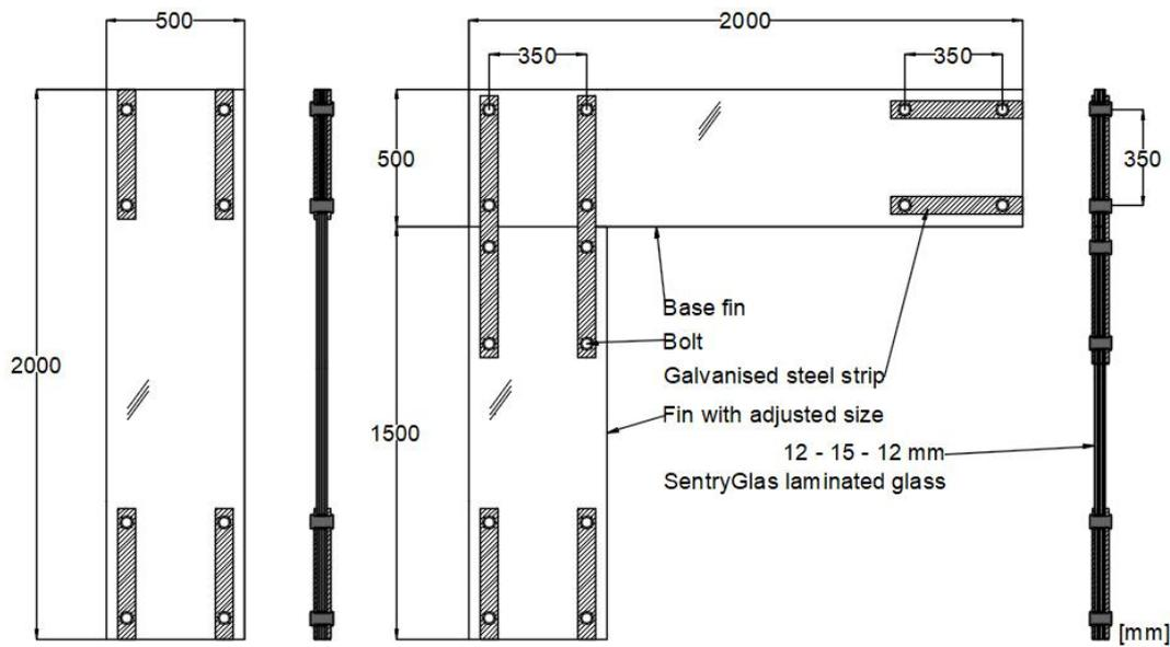
Figure 8.8: Detail of fins. Scale 1:30.
