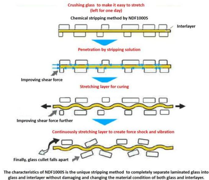
Figure 3.9: Destructive method to separate glass and interlayer. [15]
