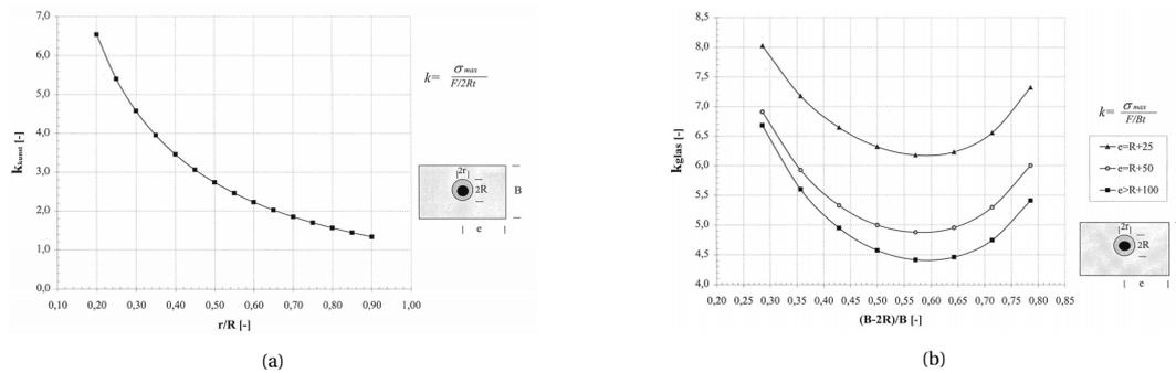
Figure D.7: Relations to derive the stresses in the glass and the filler. [38]
