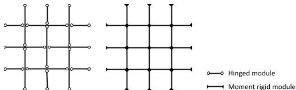
Figure 8.4: Two ways of a roof structure when continuous modules are not possible. Left: a modular structure with hinged connections built from modules with two lengths (also used in Apple Cube 1). Right: a modular structure with moment rigid connections built from a single length. Another possibility is by using continuous beams or a combination of both.
