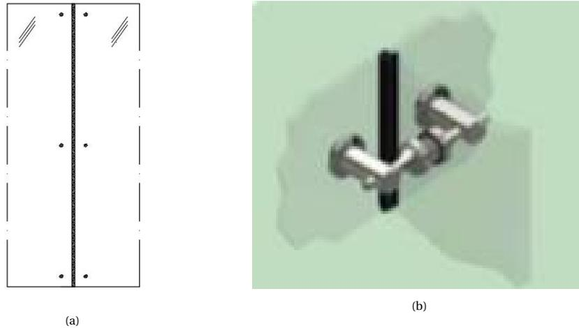
Figure E.5: Point fixing to connect facade and fin.
