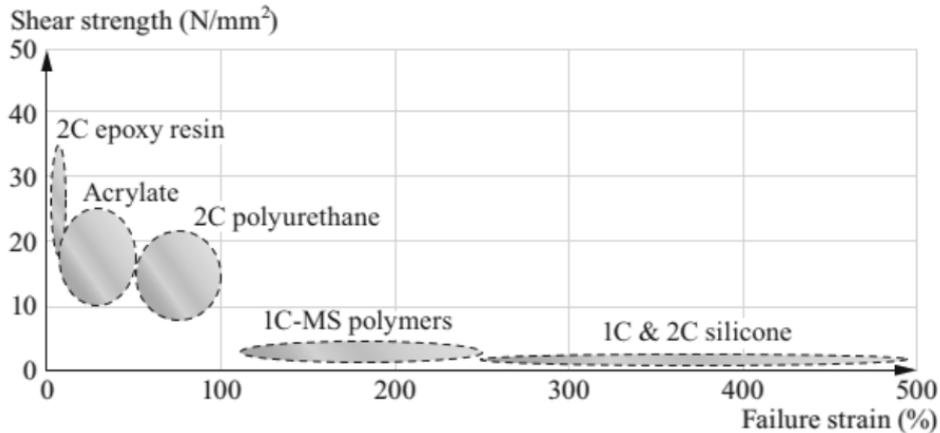
Figure 4.3: Mechanical behaviour of different adhesives [18]
