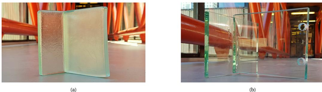
Figure 4.25: Heat bonded connections. [30]
