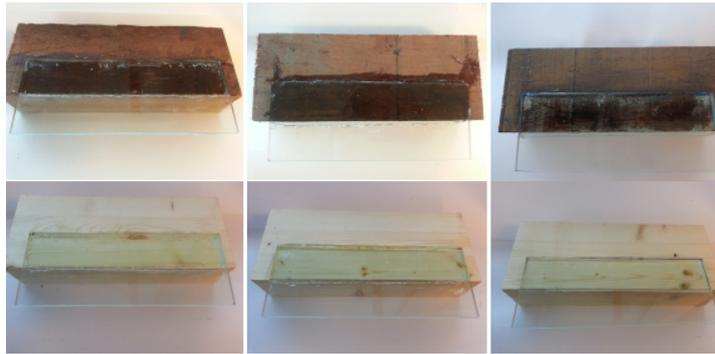
Figure 4.26: A timber to glass connection. [31]
