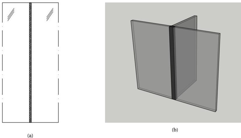
Figure E.1: Structural silicone sealant to connect facade and fin.
