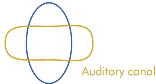
Figure 82: Example of a wrong fitting audio canal, due to the shape of the auditory canal.
