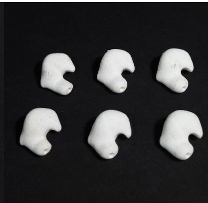
Figure 81: FDM print with new audio canal
