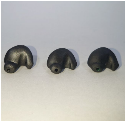
Figure 79: SLA print with new audio canal
