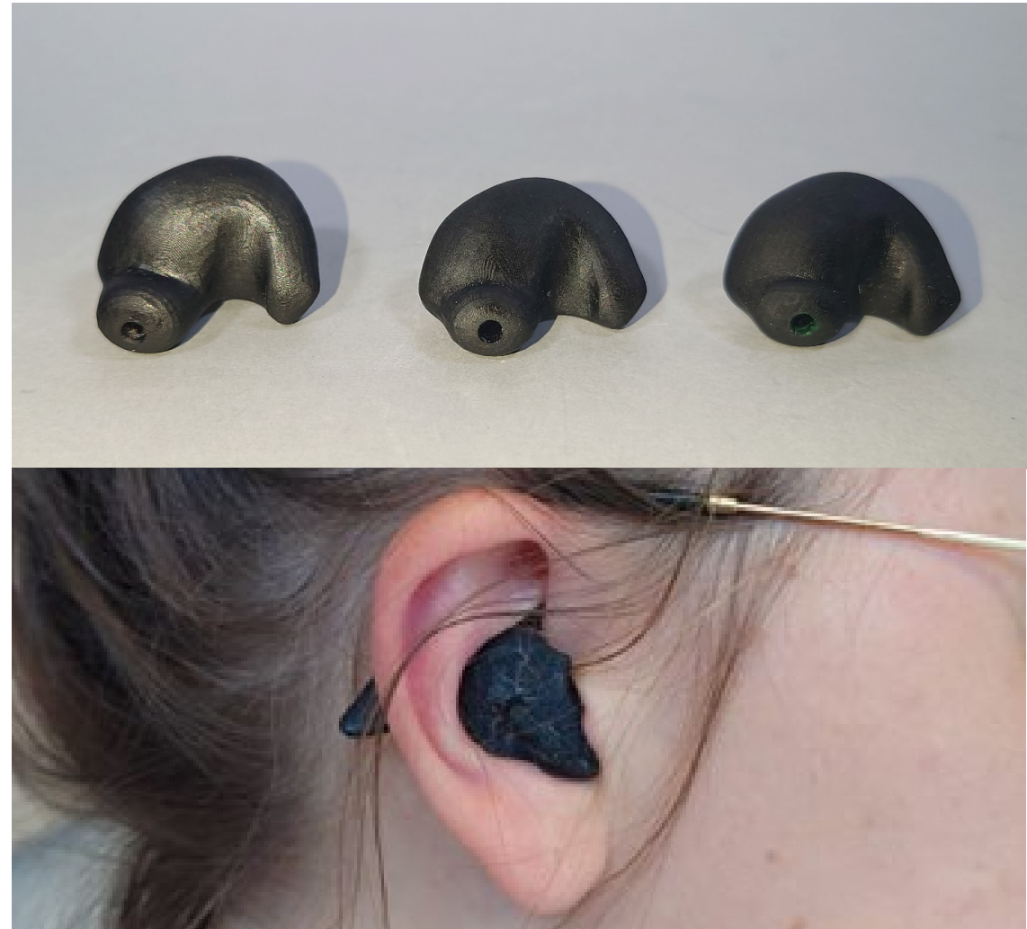
Figure 60: SLA model in the ear
