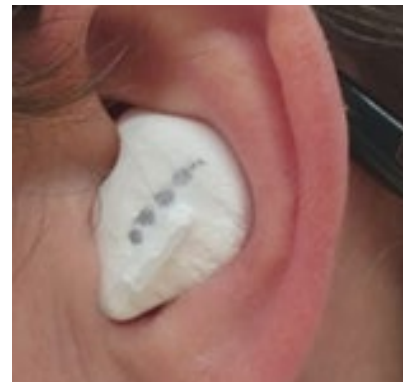
Figure 71: FDM model with a offset 0.75 mm in the ear
