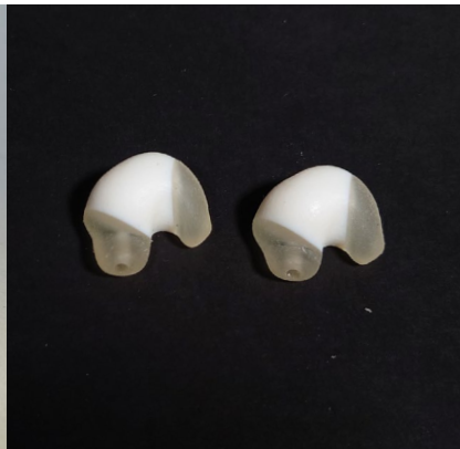
Figure 80: MJ print with new audio canal
