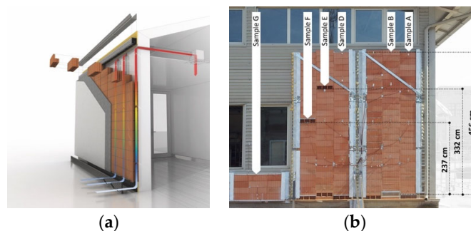
Figure 2. (a) Parietodynamic concept: Parietodynamic walls have an air cavity between the external cladding and the insulation/inner wall element. This inner element is crossed by an air duct that connects the cavity with the interior environment. The air which is transferred from the outside to the inside can be controlled according to outside and inside conditions and fans are used to force the air-flux. In this way, the supply air can be pre-tempered by solar heat gains (when the heat flux is outdoor–indoor). When this connection is closed, it acts as a regular insulation element. In summer conditions, overheating can be dissipated to some extent by enabling the energy exchange when the indoor temperature is higher than the external air temperature [45]. (b) Experimental tests of different Opaque Ventilated Facades have been carried out to characterize better the behavior of Opaque Facades under different boundary conditions [73].
