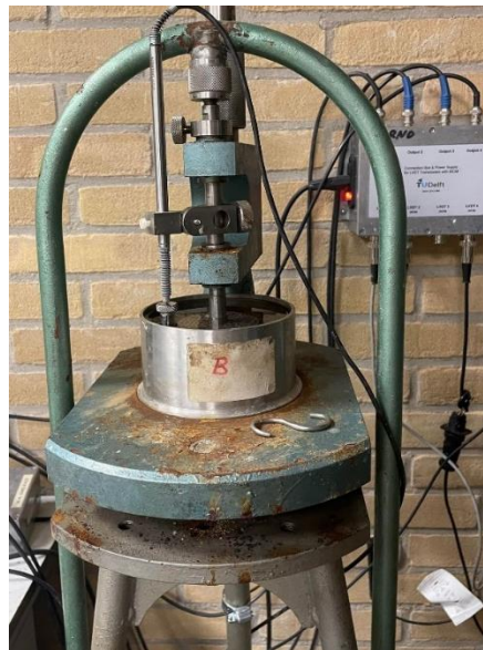
Figure 26. Incremental loading oedometer cell used to consolidate samples at TU Delft.
