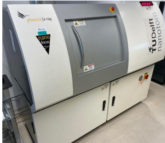
Figure 21. Nanotom TU Delft micro-CT scanner.
