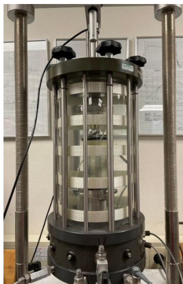
Figure 25. Bender element set-up within triaxial rig.
