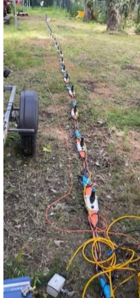
Figure 24. Multichannel analysis of surface waves (MASW) at the site in Gouda.
