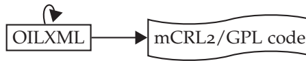
Figure 4.25: An overview of the transformation architecture of the implementation of OIL in Python. The rectangular box is an AST schema, the wavy box is text, and the arrows are transformations.
