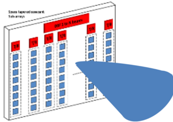
Figure 1.2: Array of vertical shaped beam sub-arrays [7]
