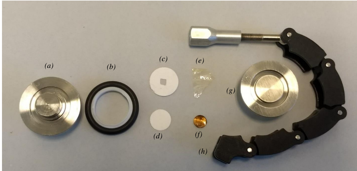
Figure 2.1: Components of a LAB Cell and the electrolytes used.
