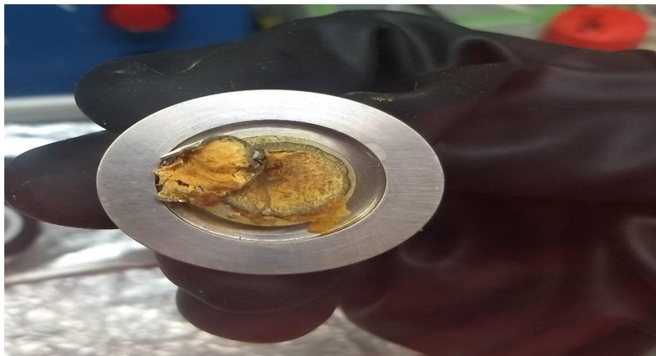
Figure 3.11: Lithium-Lithium battery with LiSPEEK Liquid Electrolyte
