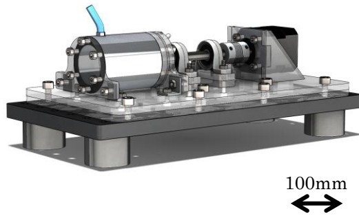
Figure 3-5: Drawing of the second experimental setup to test the ferrofluid seal with replenishing system and 10mm shaft diameter
