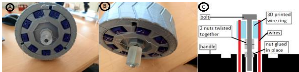
Figure 25: (A&B) Pictures of the mechanism for tightening and releasing the wires for the radial expansion mechanism. (C) A schematic of the mechanism for tightening and releasing the wires of the radial expansion mechanism.
