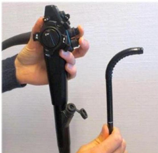
Figure 6: A State of the art flexible steerable colonoscope.
