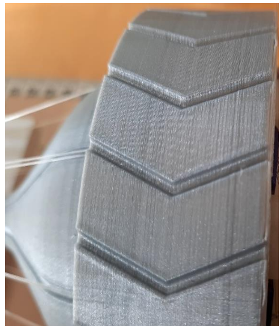
Figure 35: Picture of the cam with visible printing lines.
