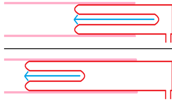
Figure 11: Schematic of a concept using a growing type of locomotion.
