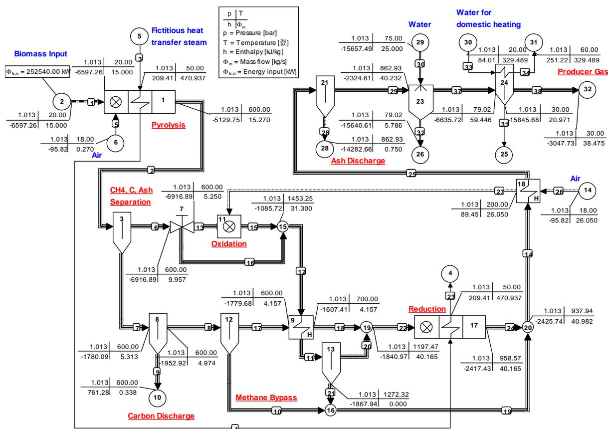
Figure 3. Three-reactor model of biomass downdraft gasifier.
