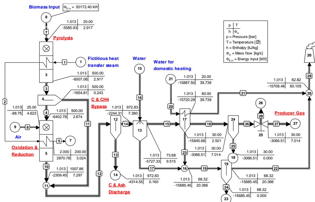
Figure 2. Two-reactor model of biomass downdraft gasifier.
