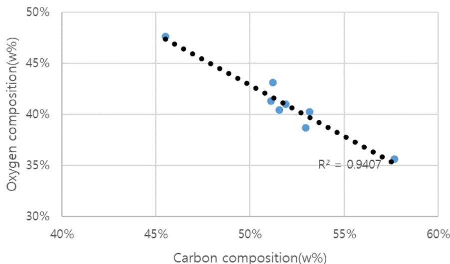
**Figure 1.** Relation between carbon and oxygen content in biomasses at dry ash free condition.
