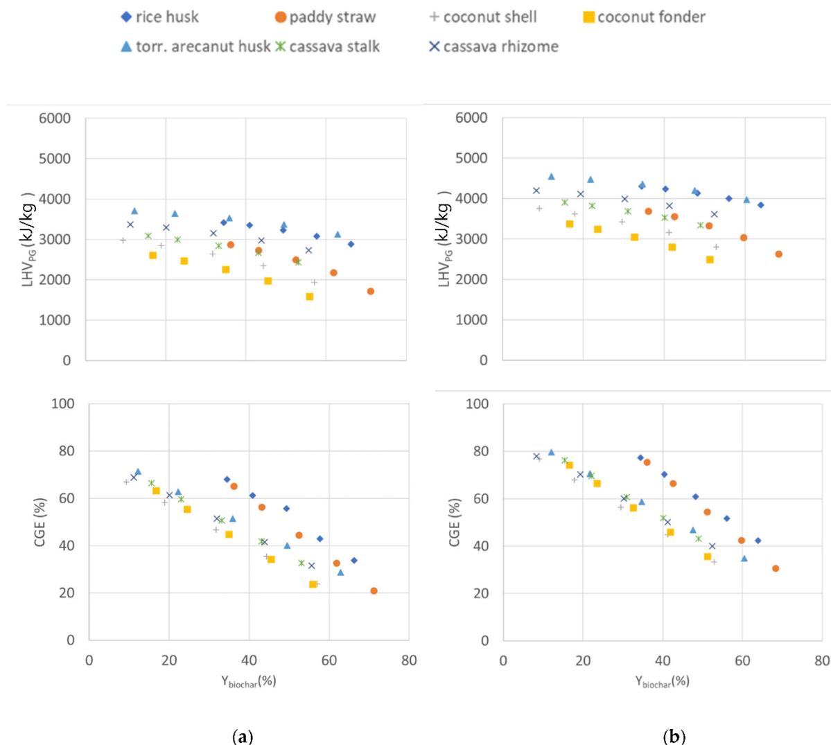
**Figure 7.** LHV<sub>PG</sub> and CGE depending on  $Y_{\text{biochar}}$ : (a) two-reactor model, (b) three-reactor model.
