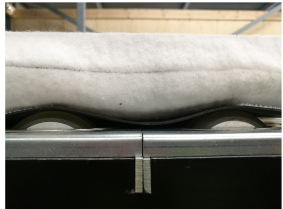
Figure 6.20: High setting for the parcel stiffness using foam stuffing which leads to a parcel which also has contact with the base plat of the IQ-Grid.
