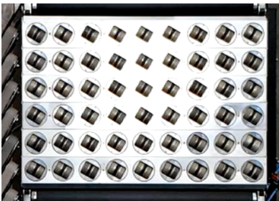
Figure 6.13: Low setting for the divert angle namely: 30^\circ which correspond with the angle of the outlet.
