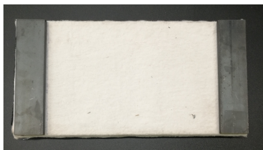
Figure 6.21: High setting for the parcel inertia by adding weight to the edges of the parcel to increase inertia, low setting is shown in Figure 6.17.
