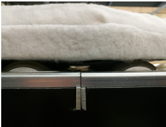
Figure 6.19: Low setting for the parcel stiffness using a MDF panel to ensure the parcel stays on top of the wheels.
