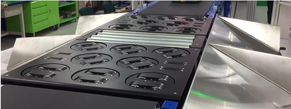
Figure C.8: Diverter using belts instead of wheels.
