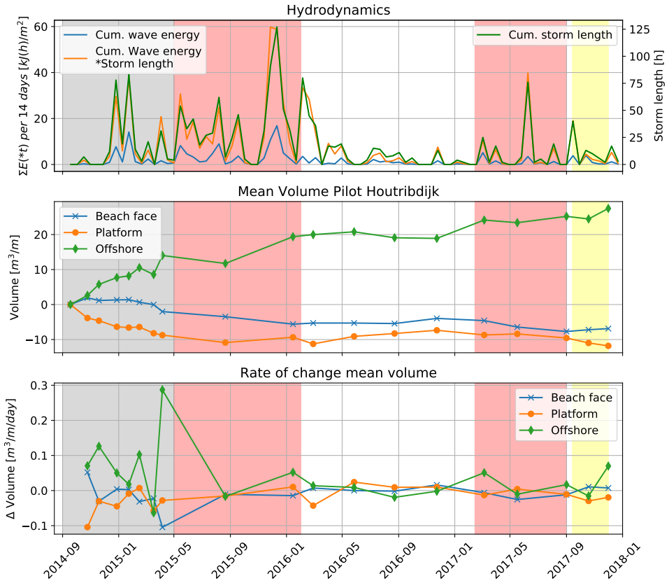
Figure 2.12: Hydro- and morphodynamics Pilot Houtribdijk. Top frame: Cumulative wave energy and average and maximum H_{m0} per 14 days. Middle frame: Volume change per section normalised to the first measurement. Bottom frame: Change to rate of volume change. Grey area: initial profile development after construction. Red areas: periods with energetic wave climate. White area: periods with calm wave climate. Yellow area: period with energetic wave climate but aberrant morphological change.
