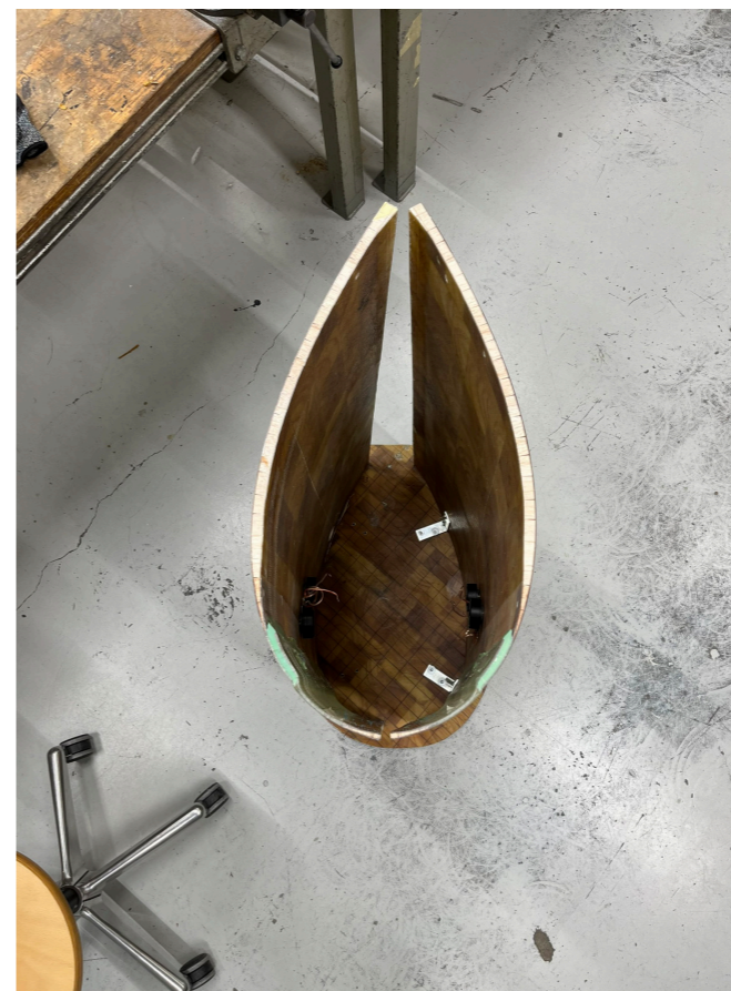
Figure 89: The main volume of the WingTone was made by bolting the curved panels to a bottom plate with L-brackets (see image on the far right).
