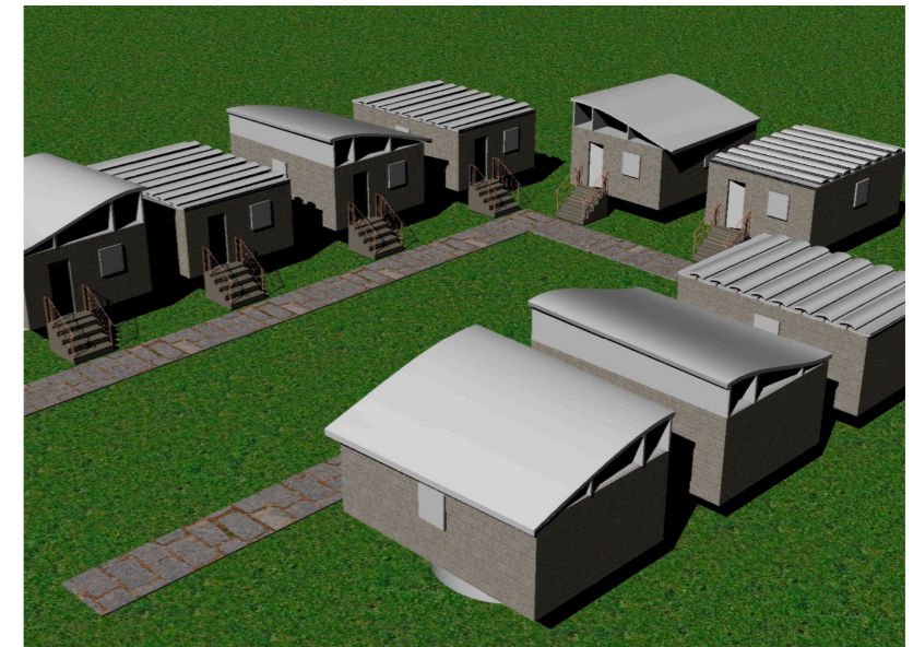
Figure 25: Emergency housing concept using WTB sections as a roof and blade root sections as structural support (Bank et al., 2018).
