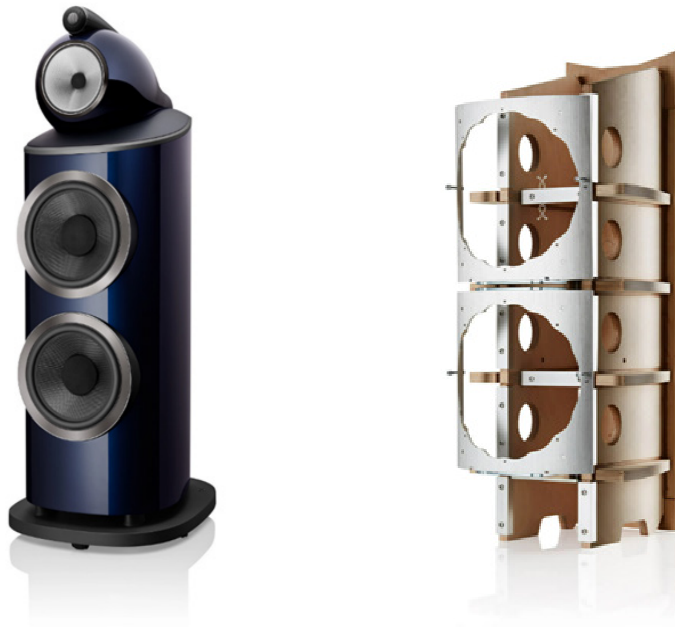
Figure 71: The Bowers and Wilkins 801 D4 Signature speaker uses internal reinforcement to decrease enclosure resonance (801 D4 Signature, n.d.).
