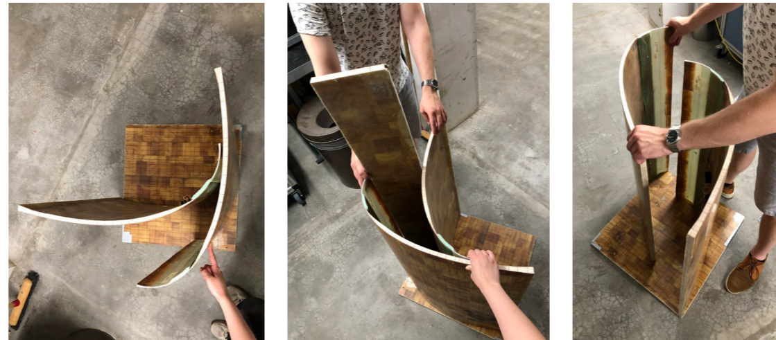
Figure 85: Quick and dirty shape exploration of generated concepts using available WTB panels.
