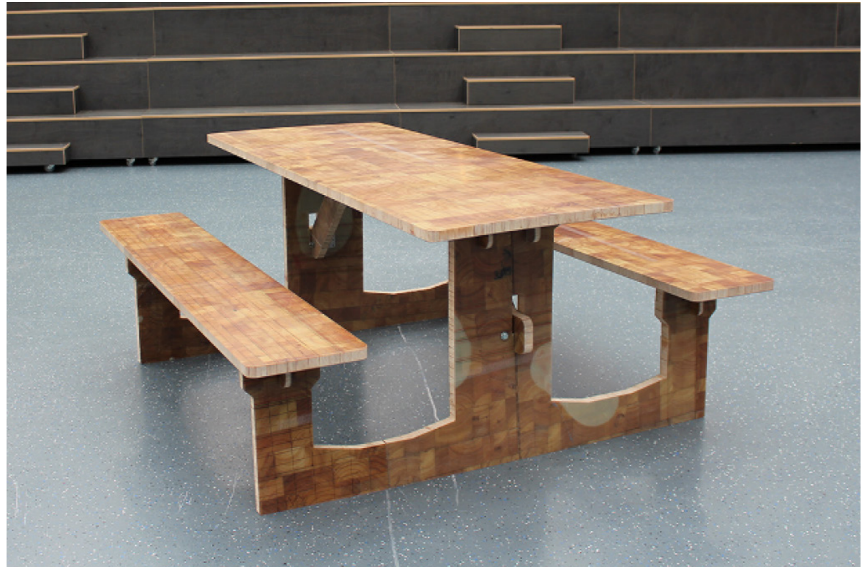
Figure 21: A rather striking example of repurposing WTBM by constructing a picnic table from sandwich material (Joustra et al., 2021b).
