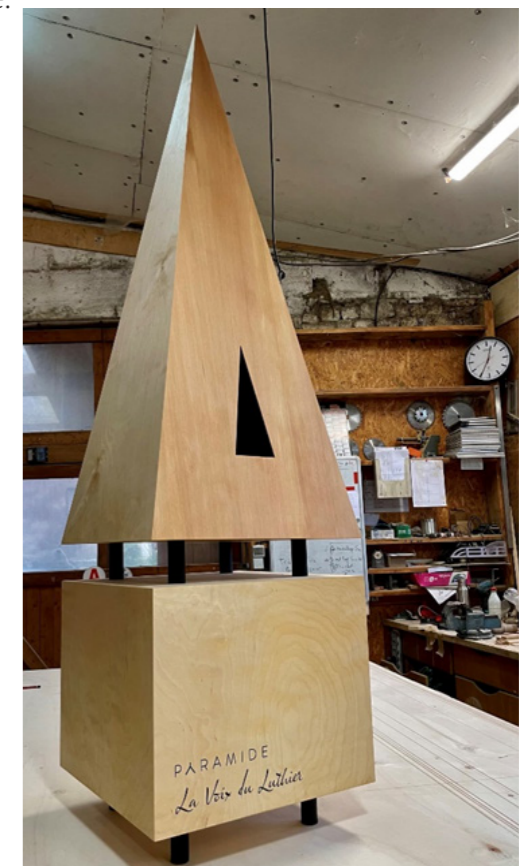
Figure 69: A resonating amplifier with a pyramid shaped cavity (La Voix de Luthier, 2023).
