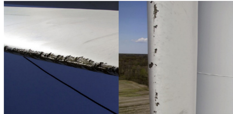
Figure 16: Examples of leading edge erosion due to wind-blown particles (Katsaprakakis et al., 2021).
