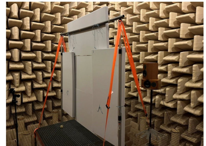
Figure 50: Test setup with a reference material (Flamex basic acoustic foam).
