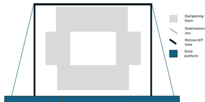
Figure 46: Diagram presenting front view of test setup without test panel.
