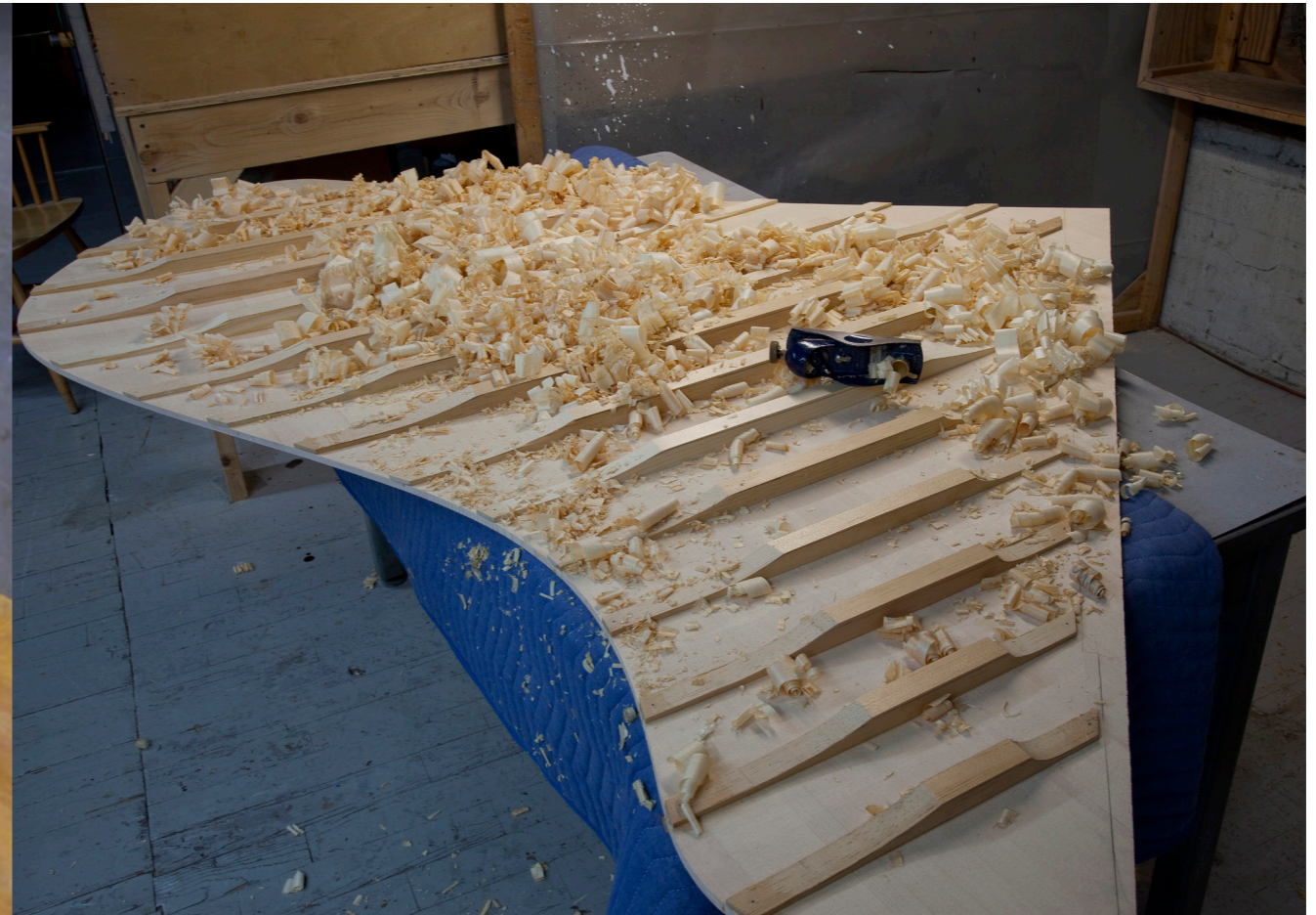
Figure 38: Grand piano soundboard made from spruce (Steinway B Sound Board Project, n.d.)
