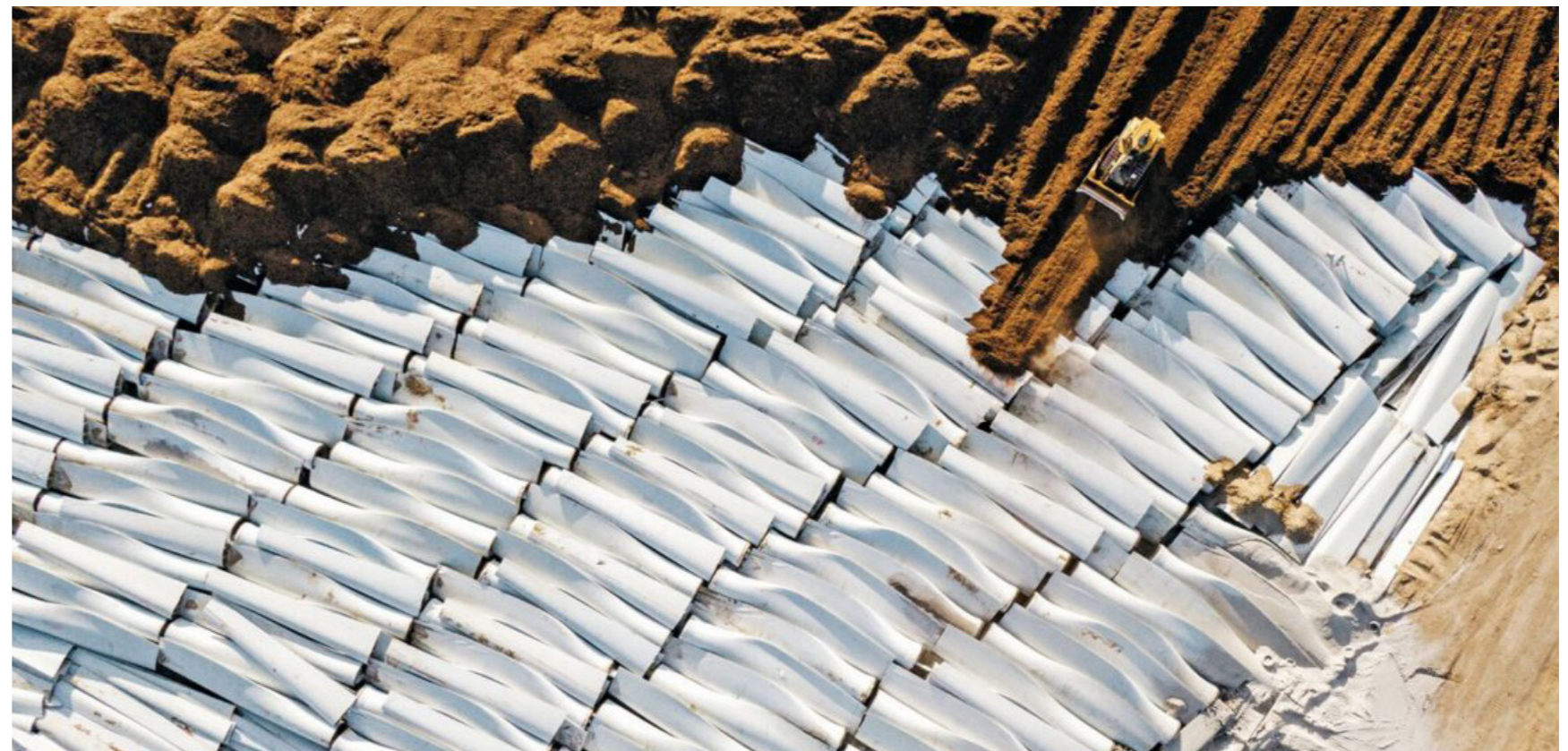
Figure 20: Scrapped wind turbine blades being buried under a layer of earth (Adobe Stock).
