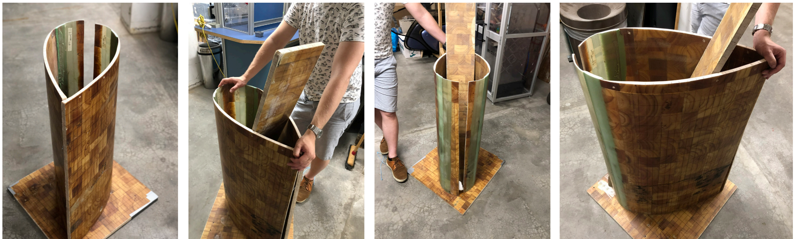
Figure 86: A promising panel configuration with an internal free-hanging panel surrounded by opposed curved panels.
