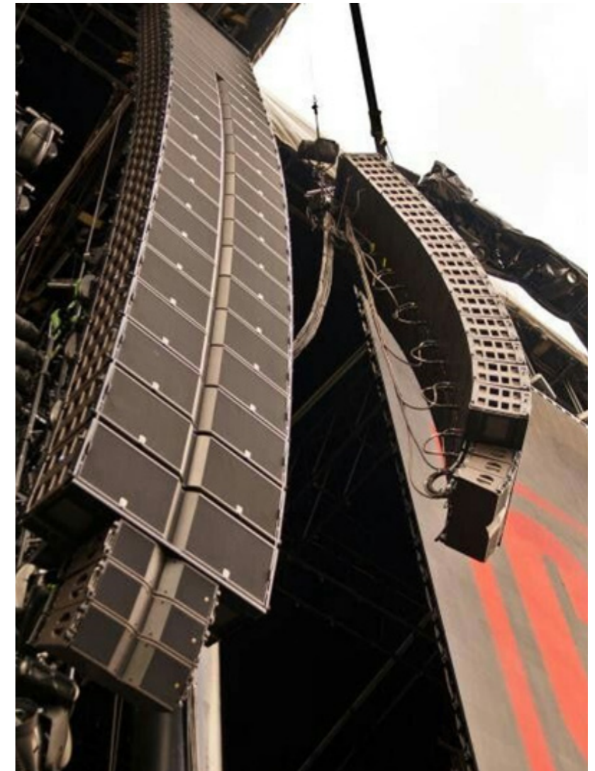
Figure 67: A line array system consisting of many modules hung up in the air, weighing more than 800kg.
