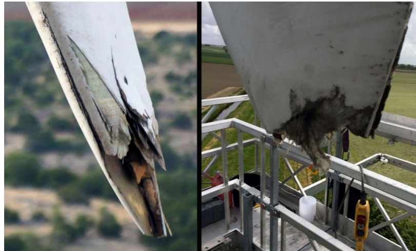
Figure 14: Shell delamination and detachment due to lightning strikes on blade tips (Katsaprakakis et al., 2021).
